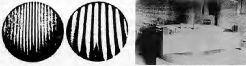
Figure 2. Left: the light-interference fringes as seen in the interferometer telescope, fringes shifted laterally as the instrument was rotated. Right: the original Michelson-Morley interferometer with an approximate 22-meter round-trip light-beam path, mounted on a concrete platform in the basement of the old Case School Physics building.
