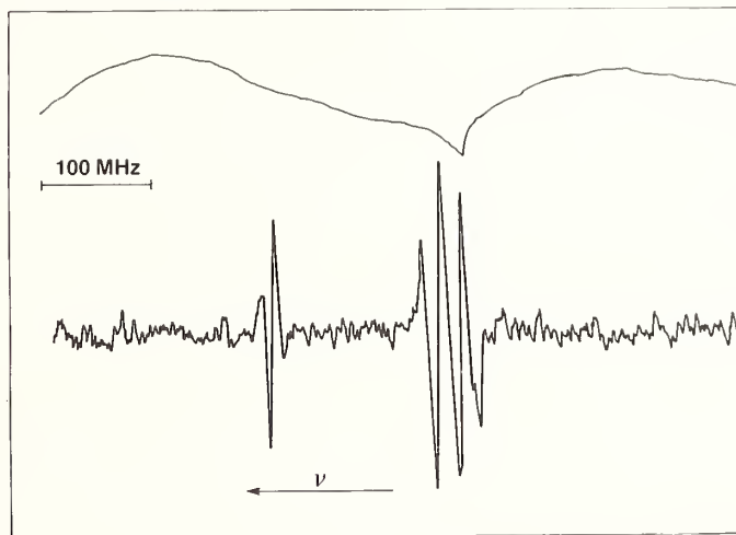
FIGURE 7. Output power and third harmonic signal vs. laser frequency for a He-Ne ( ^{127}\text{I}_2 ) laser at 0.604\ \mu\text{m} .
