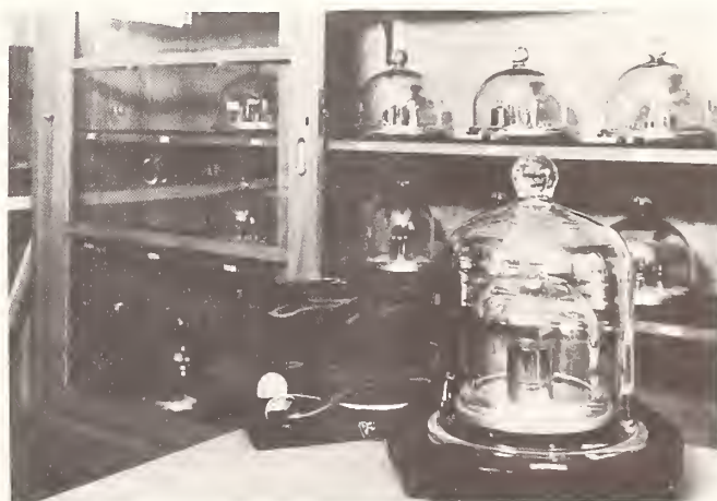
FIGURE 1. National Kilogram Prototype No. 52 at the PTB, FRG, kept under two bell-jars. In the background are further primary and reference standards.
