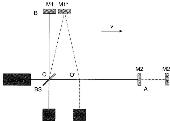
**Figure 1.** An up-to-date arrangement the of Michelson-Morley experiment. Here LASER means the source of light, BS means beamsplitter, M1 and M2 are mirrors on the end of arms, PD is the phase detector (interferometer), and  $v$  is the earth's orbital velocity, which is regarded as the inertial motion for short time periods.
