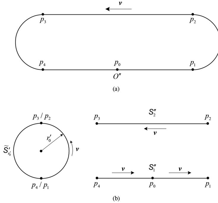
**Fig. 4.** (a) Optical fiber loop for an experiment of the generalized Sagnac effect. (b) Disintegration of the loop into circular and linear paths.
