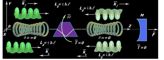
FIG. 2: (Color online) Mutual cancellation of RDS for retro-reflected photon. Rotation of the Dove prism again decreases frequency of the co-rotating forward photon with  $L_z = +\ell h$  by  $-2\ell \cdot \Omega$ . In backward propagation the Dove prism is counter rotating with respect to photon. Backward RDS is positive thus resulting  $\delta\omega$  is zero hence toroidal interference pattern is static for all  $Z$ .
