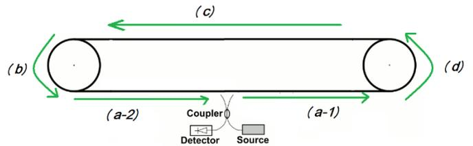
Figure 8: complete travel of the green light beam.
