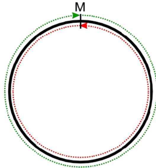
Figure 1: the interferometer is not rotating so there is not travel time difference.  $M$  is the initial position of both light beams and the detector
