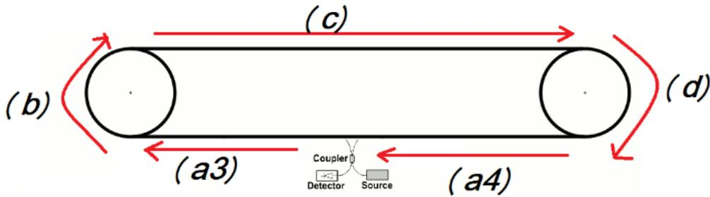
Figure 10: complete travel of the red light beam.
