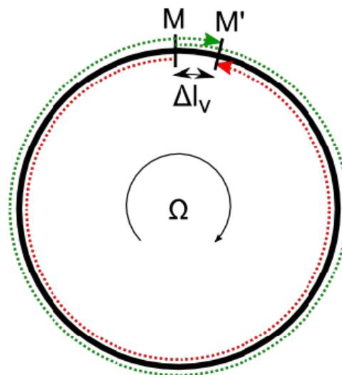
Figure 2: the interferometer is rotating at an angular velocity  $\Omega$ . The green light beam is moving with the detector and the red light beam is travelling opposite to the detector.  $M$  is the initial position of the source/detector, and  $M'$  is the final position.
