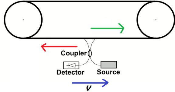
Figure 4: modified Sagnac interferometer for measured linear Sagnac effect. The initial position of the detector and the source is the same, and they move at a velocity  $V$ .
