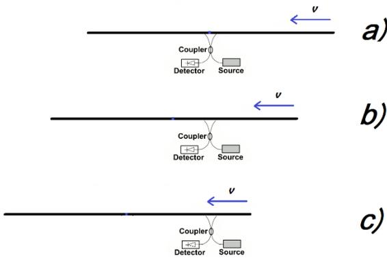
Figure 6: it is the same interferometer shown in figure 5, but the detector is stationary and the fiber interferometer is moving at speed  $V$ .
