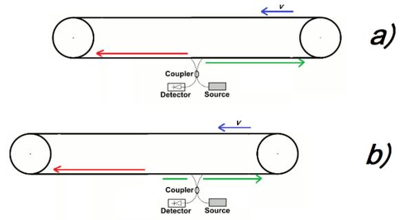
Figure 7: Same configuration shown in figure 6, but here we have the complete interferometer as in figure 4. The conveyor is moving at constant speed  $V$ . Both light beams are travelling at speed  $C$  from the detector's reference frame
