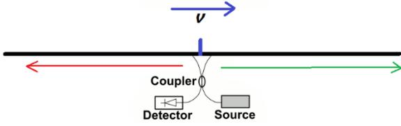
Figure 5: the detector is moving at a speed  $V$ . From the detector's reference frame, both light beams (green and red) are travelling at  $C$ .
