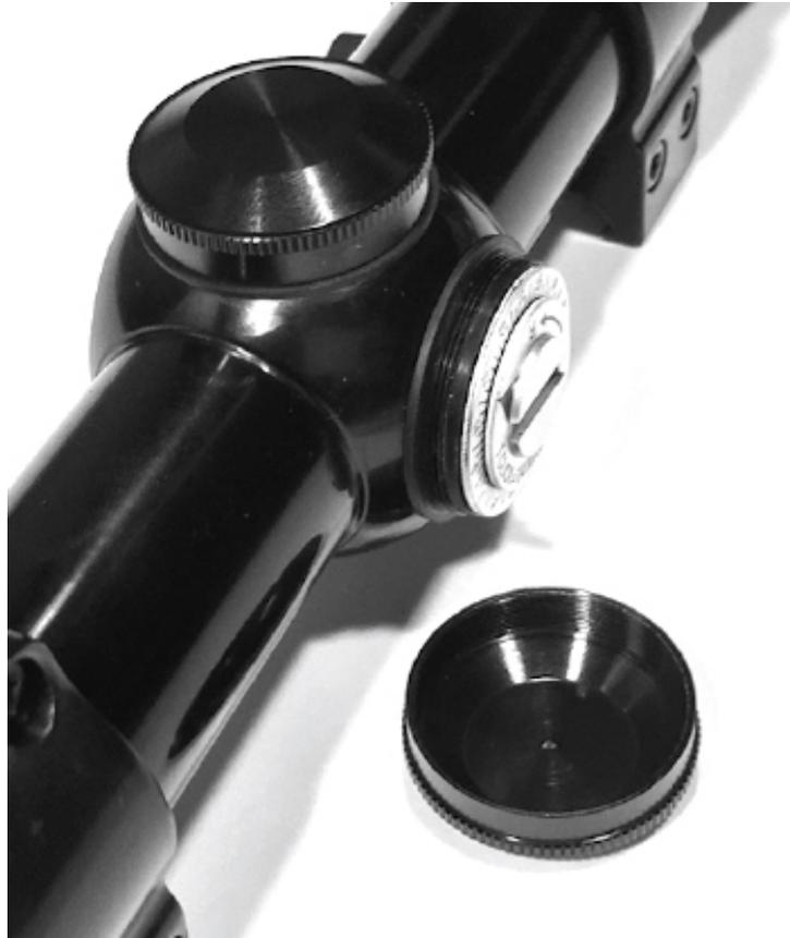
On exposed turrets, and some capped turrets, the turret itself is typically like a cap that is covering the adjustment mechanism. The turret (turret cap) is attached to the inner mechanism so that when you turn the turret (turret cap), the internal mechanism also turns. I tell people to think of the turret as a wrench that's attached to the inner mechanism like a bolt. When they turn the turret (the wrench), the inner part (bolt) also turns, so long as they're attached.
