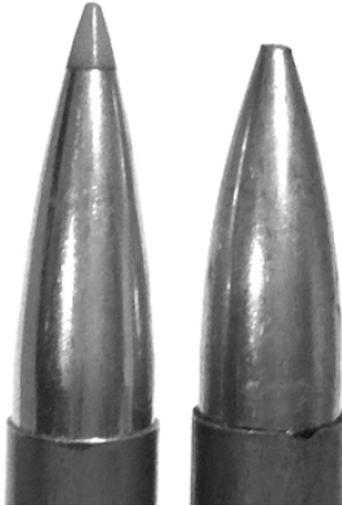
Polymer tipped bullets are a more recent trend in bullet design. A polymer tipped bullet has a larger opening than an OTM bullet and the opening is filled with a plastic tip during the manufacturing process. These polymer tipped bullets can have all of the manufacturing advantages of an OTM bullet but can also have much better consistency in tip shape.
