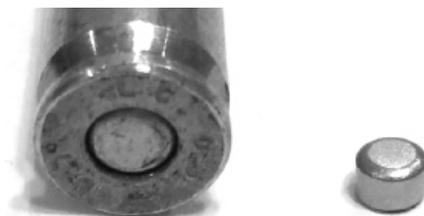
Primers are held in the primer pocket by friction alone in commercial ammunition. Military ammunition has primers which are crimped and then glued/sealed into place. Because of the friction-only hold in commercial ammunition, primers can sometimes come out of the primer pocket during firing. This is due to the pressure on the primer while the powder is burning.
