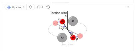
"At equilibrium (when the balance has been stabilized at an angle  $\theta$ ), the total amount of torque must be zero, as these two sources of torque cancel out:  $\kappa \cdot \theta = FL''$
