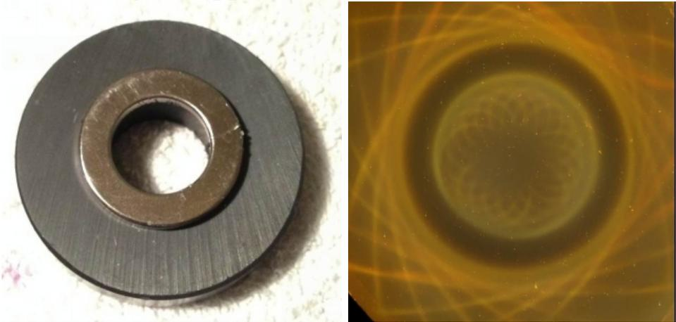
**Below: Two color inverted images of ring magnets under the ferrocell. Notice the perfect pair of inner and outer hypotrochoid of convergence and divergence.**
