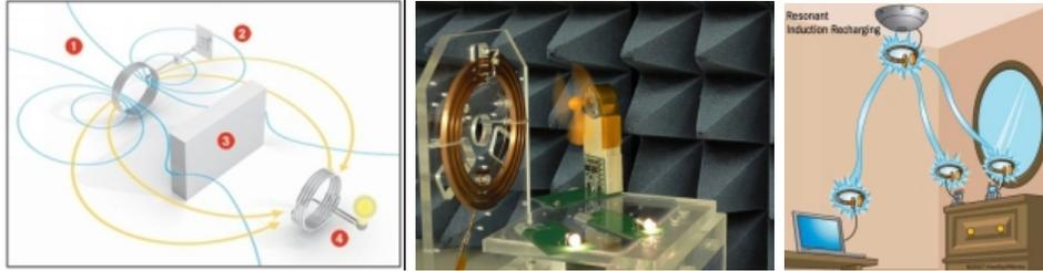
**Below and above: New developments in wireless recharging technology are being developed that will allow the charging of multiple devices at the same time without needing wires using magnetic resonance (right illustration). On the left, another company is using antennas to beam form electromagnetic energy to remote devices up to 15 feet. The powered wireless router tracks the devices and beam forms the electromagnetic energy to the device to charge it.**
