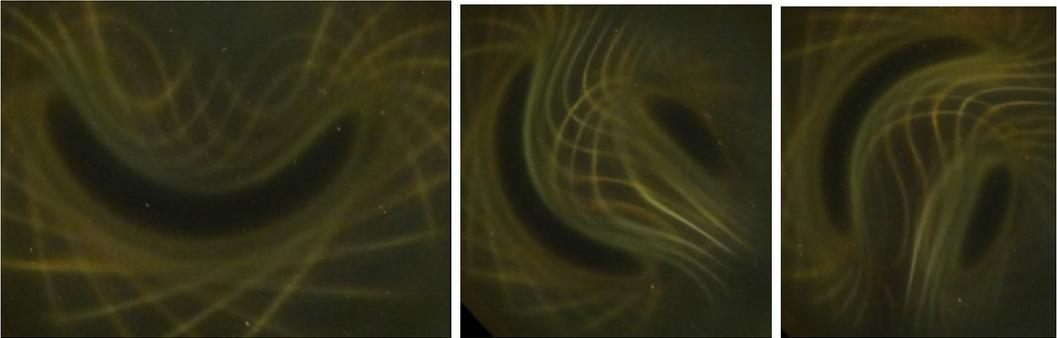
**Below: Large ceramic magnet with neodymium magnet attached. On right showing both together under the ferrocell. With field pressures equalized both magnets appear no different than a single ring magnet.**
