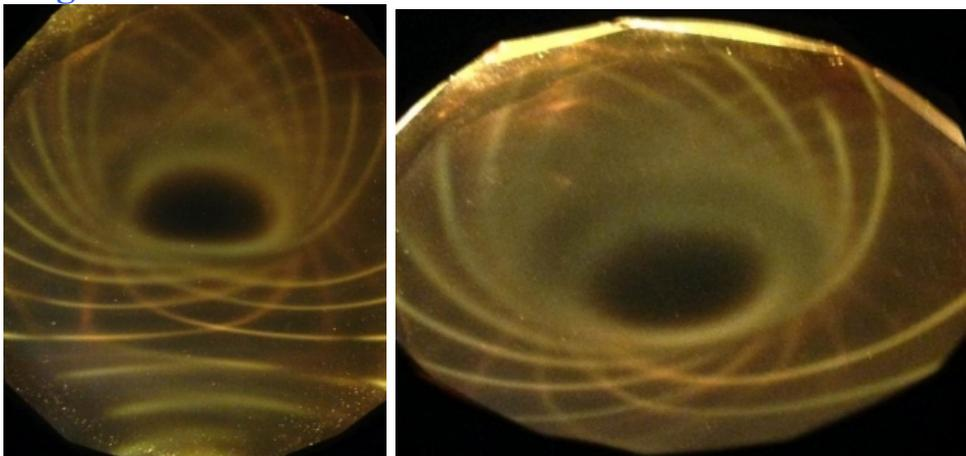
Below: Three images of cube 1” magnets under the ferrocell. Notice the bright white light along the inertial plane on the images, especially on the far right.
