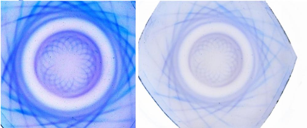
**Below: Cube magnet under ferrocell. Polarity is left to right on left image, and top to bottom on right image. Notice the brighter yellow light along the inertial plane of the magnet.**
