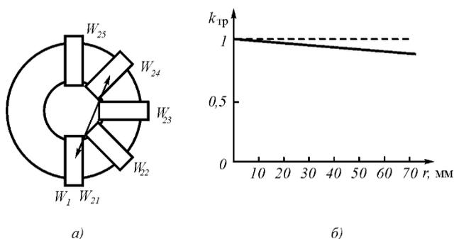
**Fig. 3.2. Dependence of the relative value of the transformation coefficient on the winding arrangement:** *a* - scheme of winding arrangement on the ring core during the experiment; *b* - change of the transformation coefficient when the distance between the windings is changed.
