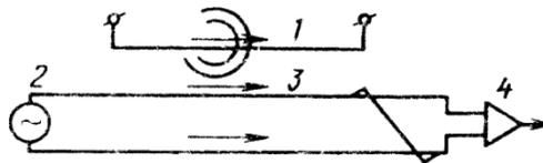
Fig. 1.8. Interaction of electromagnetic flooding with bifilar water: 1 - source of flooding; 2 - source of signal; 3 - communication line; 4 - differential receiver.
