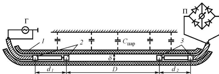
**Figure 6.4. Schematic diagram of the experiment to test the longitudinal propagation of radiation of a dipole with concentrated parameters:**
