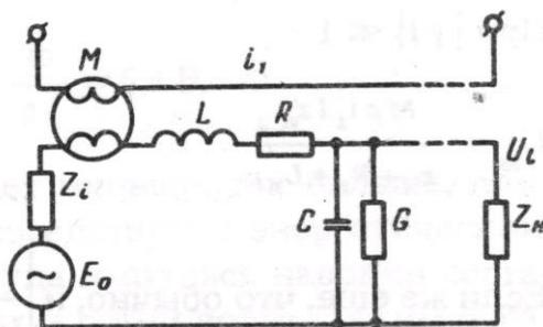
**Fig. 1.5. Equivalent scheme of electromagnetic coupling of circuits:**  $M$  - coefficient of mutual inductance;  $i_1$  - current in the primary circuit;  $U_p$  - interference voltage in the secondary circuit;  $L, R$  - specific distributed inductance and resistance of the secondary circuit;  $C, G$ , capacitance and conductivity of losses of the secondary circuit;  $E_0$  - useful signal;  $z_i$  - internal resistance of the source of useful signal;  $z_n$  - load resistance.
