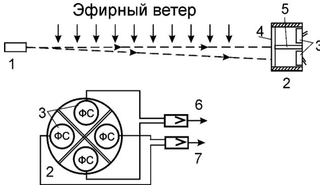
**Fig. 1. Scheme for measuring the ether wind velocity using a laser beam:** 1 - laser; 2 - detector; 3 - photoresistance; 4 - matte glass; 5 - opaque partition; 6 - amplifier of the beam vertical deflection signal; 7 - amplifier of the beam horizontal deflection signal.
