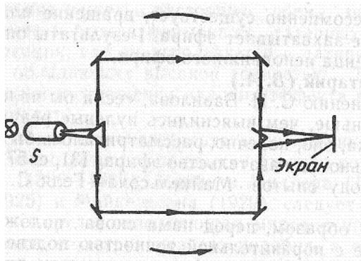
**Figure 3.5. Schematic diagram of the experiment to reveal the Sanyak vortex effect**
