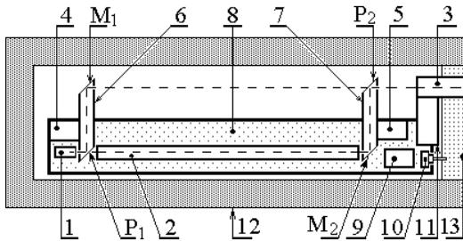
**Fig.5. Interferometer design**
