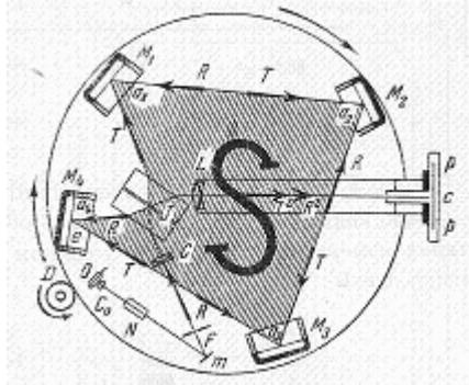
Figure 3. 8. Sanyak interferometer
