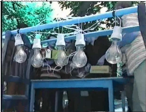
**Figure 9. Five one-kilowatt load lamps**
