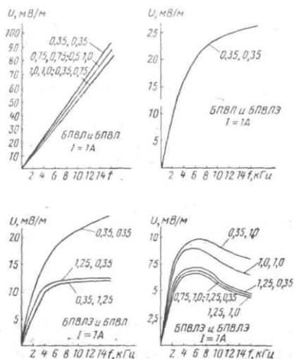
**Fig. 1.6. Results of experimental determination of interconnection of BPVL and BPVLE wires of different cross-sections (wire cross-sections are given in mm ).<sup>2</sup>**
