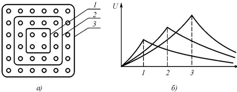
**Fig. 4.3. Change of EMF on measuring circuits as the number of connected current-carrying circuits increases:** *a* – arrangement of measuring circuits on a plate with current-carrying coils creating a magnetic field; *b* – EMF on a measuring circuit as current-carrying coils are connected.
