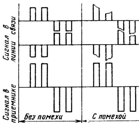
Fig. 1.9. Separation of the useful signal from the interference in the differential signal receiver with the use of RZ-code ("return to zero")
