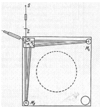
**Fig. 3.11. Schematic diagram of the Kennedy interferometer**
