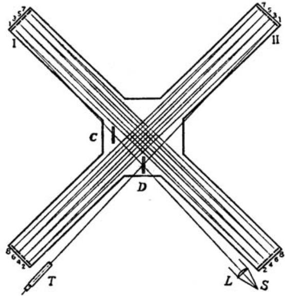
FIG. 4. **Light Paths of the Michelson-Morley and Miller Interferometers**, as seen from above. Source (S) generates light which passes through lens (L) and is then split by half-silvered mirror (D). Beams then reflect back and forth along beams (I and II) to mirrors (numbered 1-8) before finally being recombined by half-silvered mirror (D) and reflected to small telescope eyepiece (T) where interference fringes are observed.
