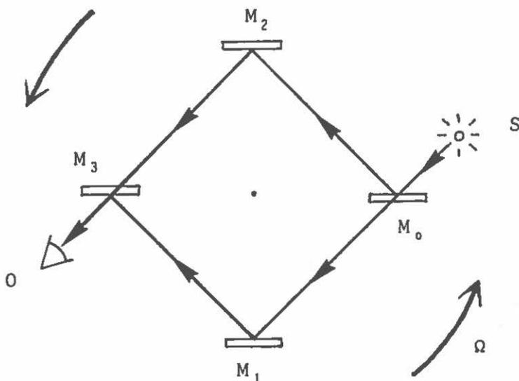
Fig. 1. The oneway Sagnac device where light travels essentially in one direction only (from right to left for the orientation shown).
