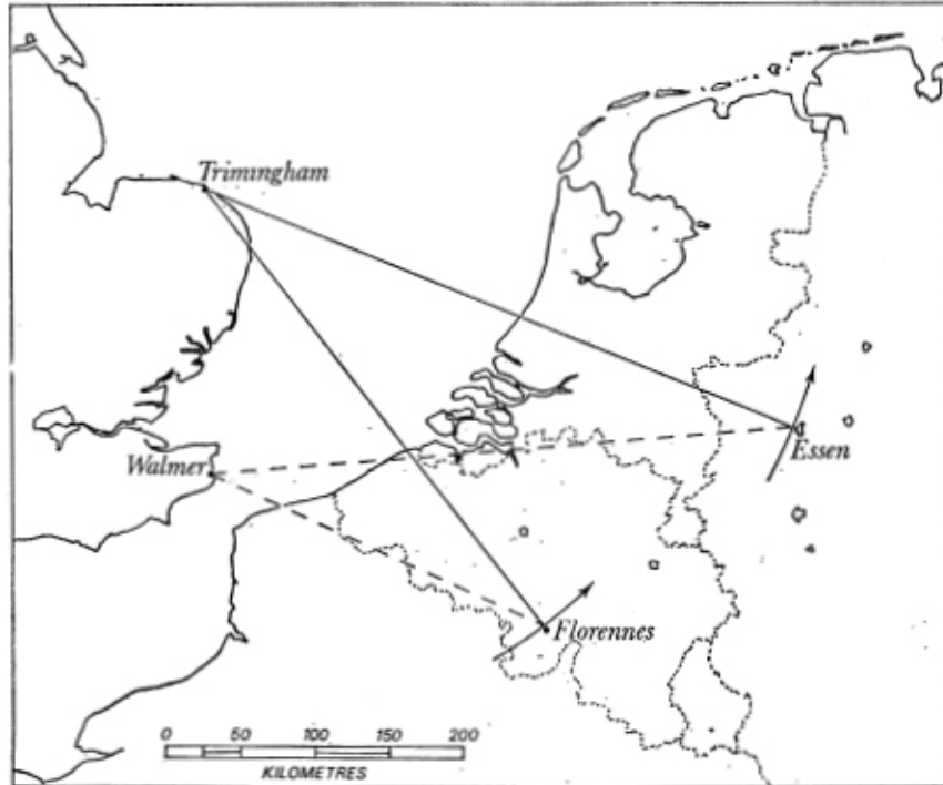
Fig. 15. The 'Oboe' dispositions for bombing Florennes and Essen. The bombing aircraft flies at a constant range from the ground station at Trimingham, taking it on an arc. When it is at the correct range from the ground station at Walmer, the latter sends the order for bomb release. The curved tracks are slightly (but exaggerated in the diagram) to the west of the targets because the bombs continue on a tangent after release
