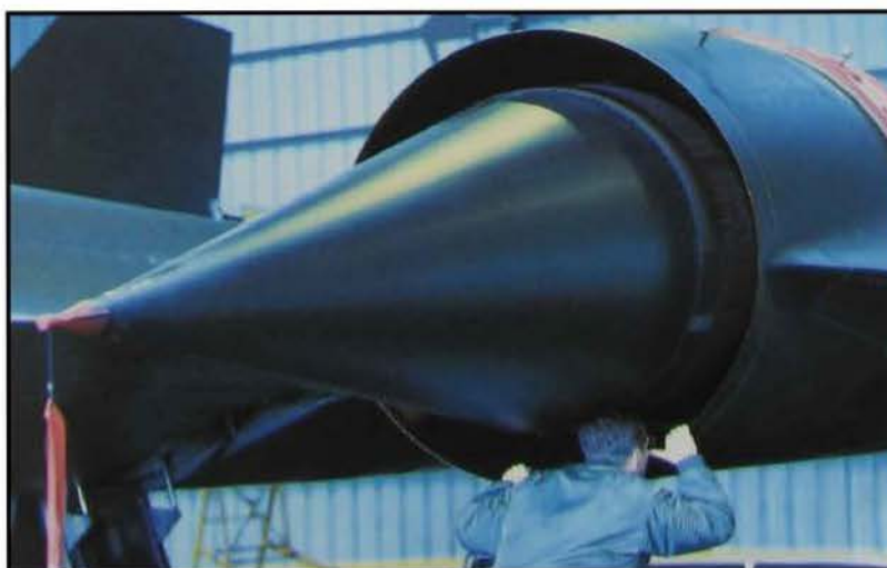
Long before the crew arrived, maintenance was doing its job. Here the large intakes are being inspected. The sharpness of the spike warranted tip covers.
