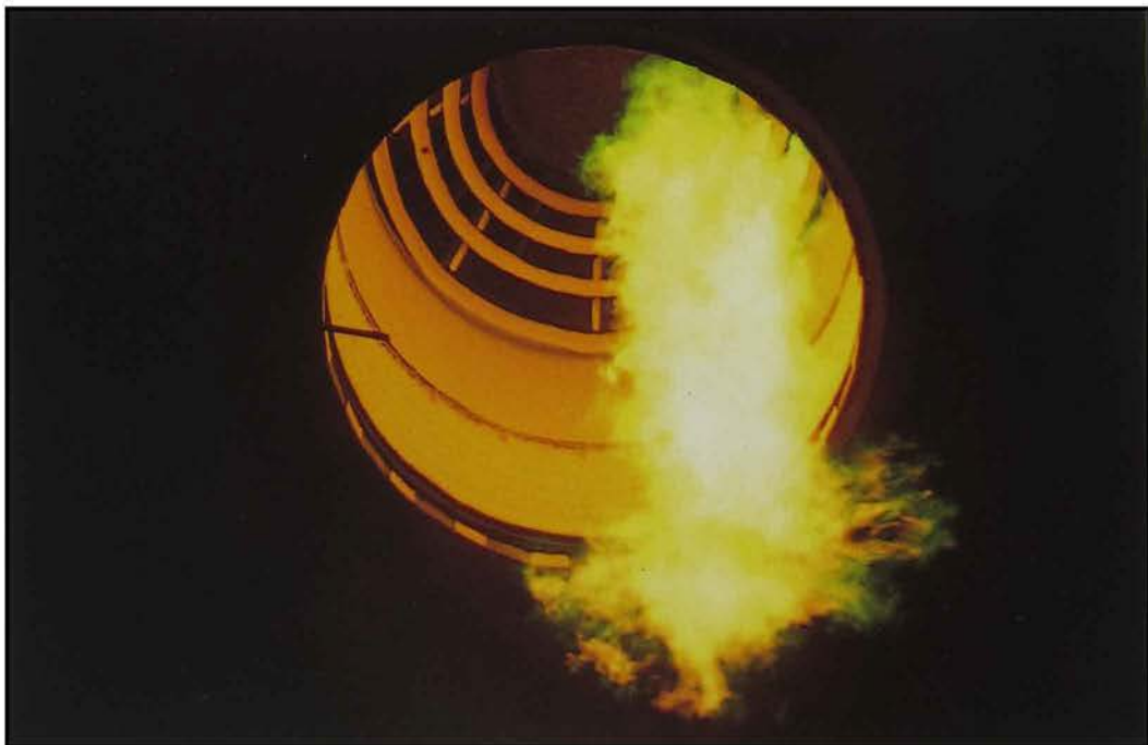
Tetraethyl Borane ignites JP-7 and with a burst of flame an SR-71 engine is started.
