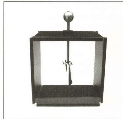
A simple, commercially available leaf electroscope.
