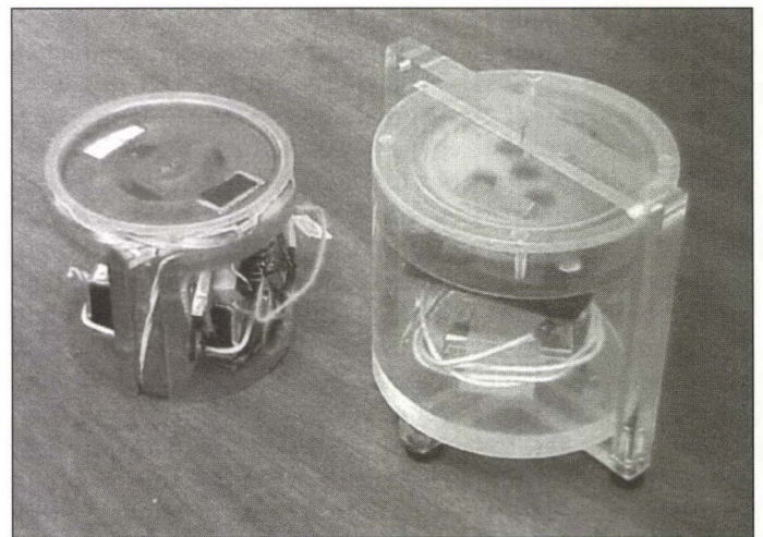
Photo 1: The KLP motor stator and internal rotor are on the left. The stator contains the 300 turns of 34 gauge magnet wire coils, bundled with rubber bands, and two batteries with switching circuitry, as the KLP motor is an opto-electronically commutated DC motor. Inside the stator housing and on top is the rotor, containing two rectangular magnet stacks; one stack has a black tape marker on it. The body pieces of both motors are made of polycarbonate. The conventional motor is on the right, made from a 12VDC fan; the fan blades were cut off and the rotor with the magnets was glued on. The conventional motor is inside the frame and inside the rotatable stator outer jacket, used to hold the stator and to reduce windage. Its rotor is nearly the same mass and moment of inertia, and was operated at the same speed as the KLP rotor, when this latter and its stator assembly were inside the rotatable stator outer jacket.
