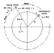
The relative motion between the USNO located and the flying clocks would create a time shift between them. Starting then from the general GR expression, the differential expression for the metric in the moving frame with respect to the one in the fixed frame is
