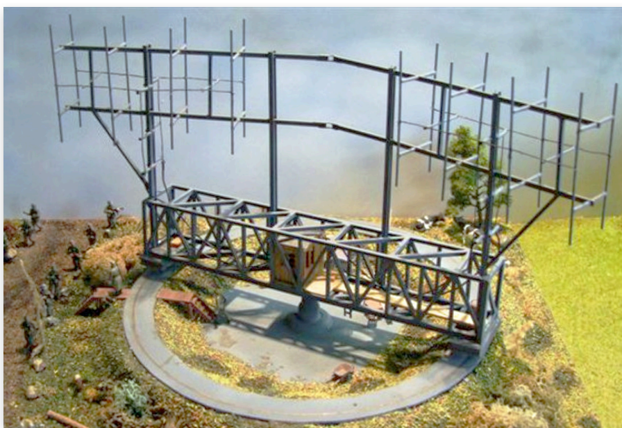
After the occupation of the Netherlands and France, more compact second-generation 45m-wide FuSan721 Knickebein antennas could be used, as they could be sited nearer to Britain. (Model by Michael Kayser)
