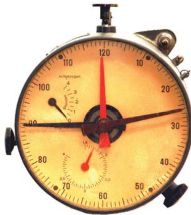
The X-Gerät 'bombing-clock' measured the time to fly between two crossbeams to determine the bomb release time. (Horst Beck Collection, photo Frank Dörenberg, N4SPP/F4WCN).
