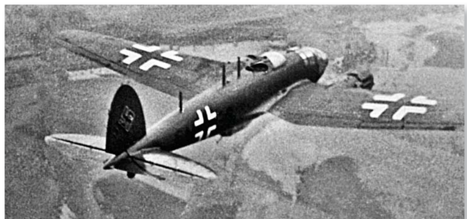
The three dorsal antenna masts reveal that this Heinkel 111 was an X-Gerät pathfinder.
