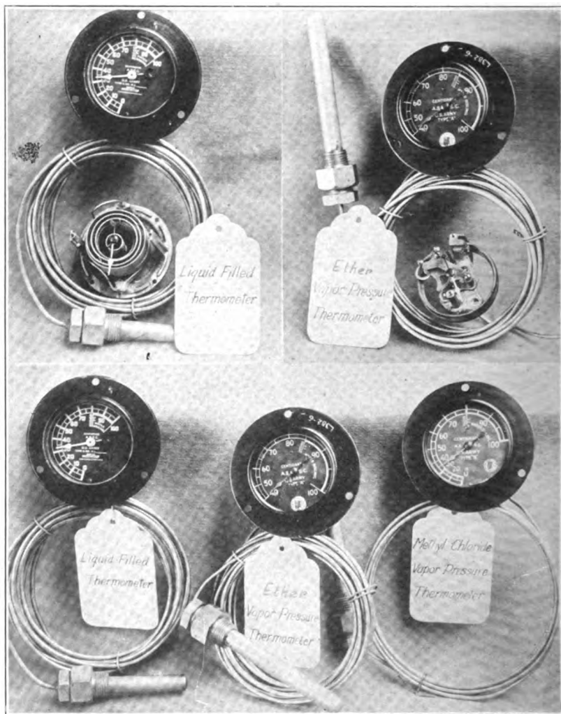
FIG. 24. Liquid and Vapor Pressure Thermometers
