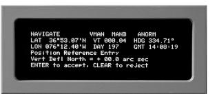
If Vertical Deflection North displays 00.0 arc seconds, press the **<ENTER>** key. If it does not, press the **<CLEAR>** key. Enter +00.0.
