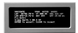
(b) To enter a different value, press the **<CLEAR>** key and enter fix Sigma North (SN) in xx.x NM format.
