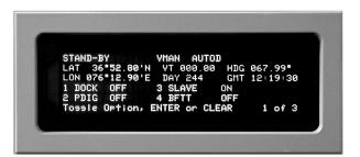
(2) Coarse ALIGN (Dockside) - To select Dockside Alignment, select DOCK ON on Page 1 of the Sensor menu, then enter a time and position fix within 0.01 nm accuracy. While Coarse Align in Dockside is being performed, the words ALIGN and DOCK appear in the upper-left fields of the display.
