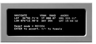
Take a position fix using the best available reference, usually a GPS fix. Take a mark of position and note the exact GMT of the mark.
