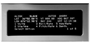
c. Upon completion of Coarse Align, verify ALIGN-C appears in the upper-left field of the display, indicating performance of Fine Align.
