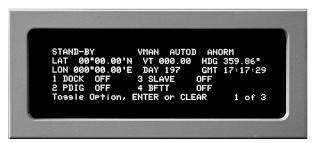
Select DOCK ON, PDIG ON, or SLAVE ON and m. press the **<ENTER>** key to select Align mode.
