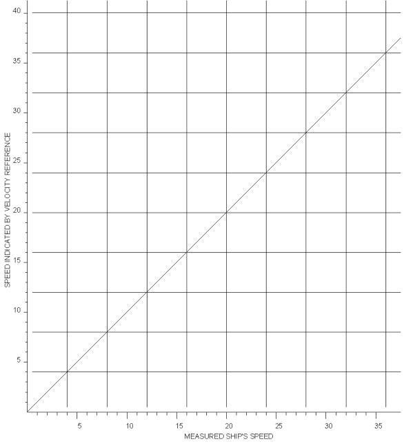
Figure 8-13. Sample Speed Bias Calibration Worksheet
