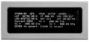
Press the **<ENTER>** key again to accept the GPS as the Digital Velocity source. The system will display notification that it has accepted the velocity reference.
