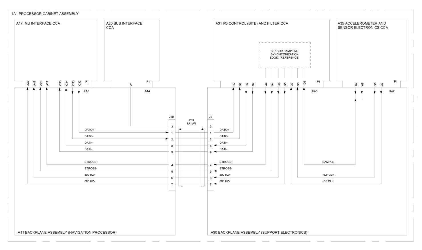
Figure 5-19. Parallel Bus Data, Address and Control Functions, Distribution Diagram (Sheet 4 of 5)
