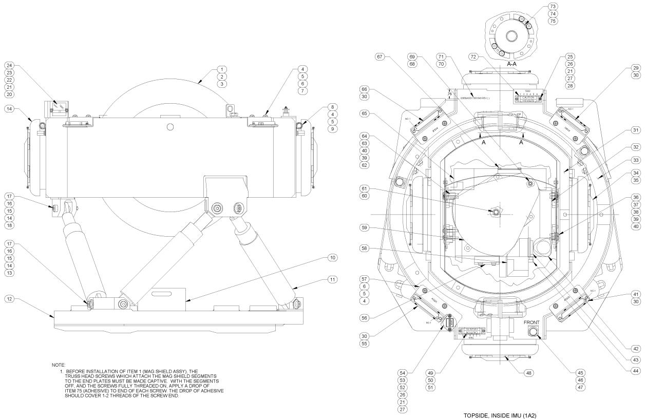
Figure 7-8. IMU: Subassembly Identification (1A2A1A1)
