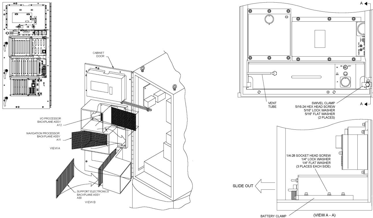
Figure 6-4. Removal of Backplane Wiring Assemblies
