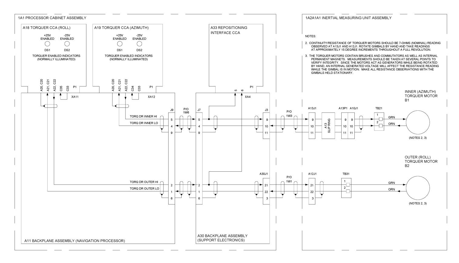
Figure 5-13. Roll (Outer) and Azimuth (Inner) Gimbal, Synchro and Torquer Loop Diagram (Sheet 2 of 2)
