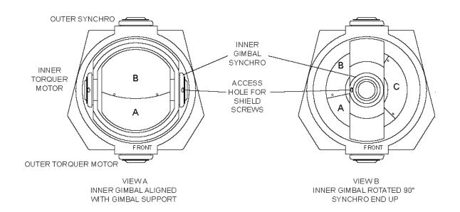
Figure 6-11. Mounting of Magnetic Shield on Sensor Block Assembly (1A2A1A1A9)
