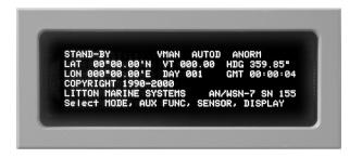
The unit will remain in STANDBY until the first valid position fix is accepted (either manually entered or from an external position reference source).
