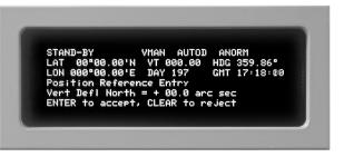
c. Press the **<ENTER>** key to accept the Vertical Deflection North Value. The display will show the "Vertical Deflection East" with a value of 00.0 arc sec and prompt the operator to accept or reject it.
