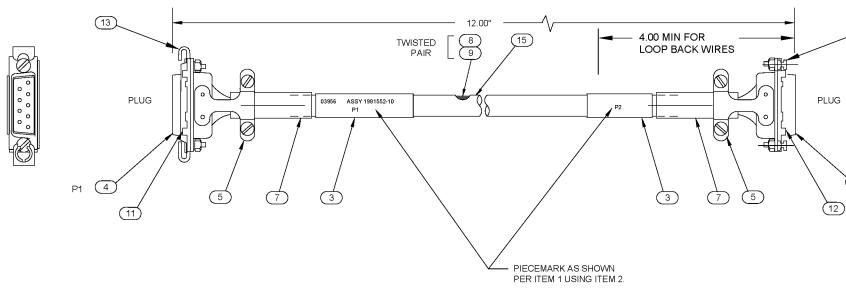
Figure A-4. IMU Interface BIT Test Cable 1981552-10
