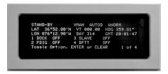
b. Press the **<SENSOR>** key and select PDIG ON.
