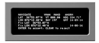
If the displayed position is correct, press the m. **<ENTER>** key again. The RLGN checks the entry for reasonableness and accepts it.
