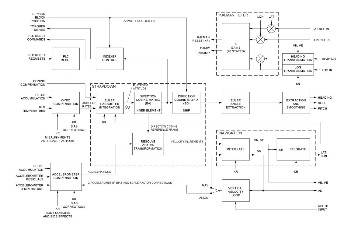
Figure 3-10. Strapdown Processing Block Diagram
