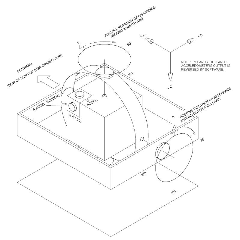
Figure 3-19. Platform Indexing Orientations
