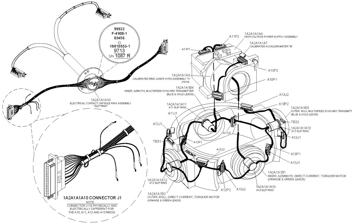
Figure 6-15. Location of Slip Rings in Inertial Measuring Unit
