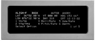
(5) NAVIGATE (Selected from Dockside or Slave) - If the system has been selected to align at Dockside or Slave, the Fine Align (ALIGN-F) mode remains active until the Navigate mode is manually selected by the operator.
