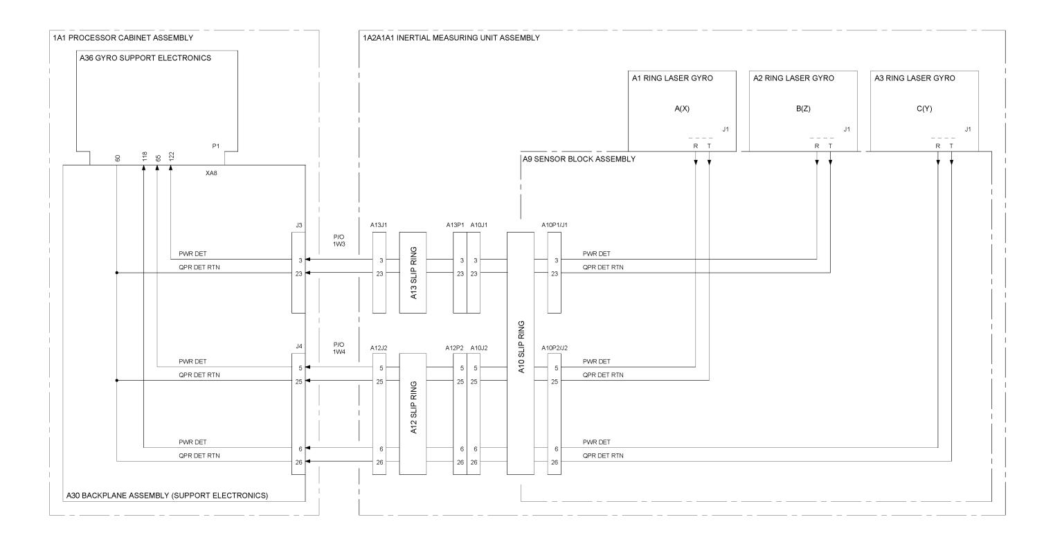
Figure 5-14. Ring Laser Gyros, Path Length Control and Random Drift Improvement Control Functions Diagram (Sheet 2 of 2)
