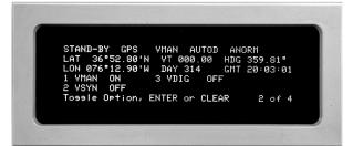
K. To select the GPS as the velocity reference, press the <3> key.
