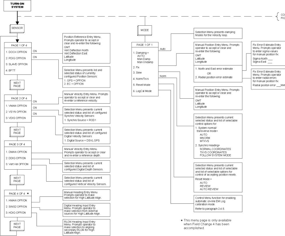
Figure 2-4. Identifying Operation Menus and Data Entry (Sheet 1 of 2)
