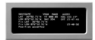
**2.3.4.12 Review Reset Data Procedure.** You can review reset data for the most recent fix, including fix data, type of fix (manual or GPS), and date and time of fix.
