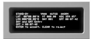
k. Press the **<CLEAR>** key to reject the GMT entry and enter the correct time. Press the **<ENTER>** key to accept the entry. The display will show the Julian day and GMT.
