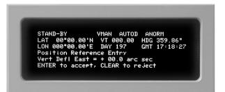
d. Press the **<ENTER>** key to accept the Vertical Deflection East value. The display will show the latitude and prompt the operator to accept or reject the latitude value.
