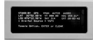
m. If VGPS is not displayed, press the <1> key to toggle the options until VGPS is displayed as the Digital Source and press the <ENTER> key. The display will show the current GPS North, East, and Vertical velocities.
