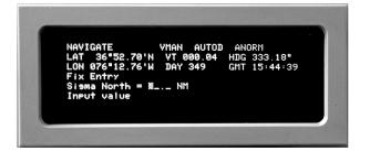
Press the **<ENTER>** key to accept the entry. The display will now prompt for entry of fix Sigma East (SE). Current Sigma East (SE) is displayed and may be accepted by pressing the **<EN-TER>** key.
