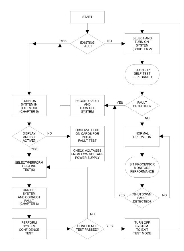
Figure 5-1. Maintenance Turn-On and Test Selection Sequence
