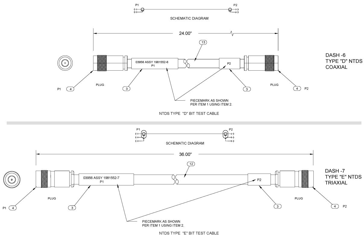
Figure A-2. NTDS Type D and E Interface BIT Test Cable 1981552-6 and -7
