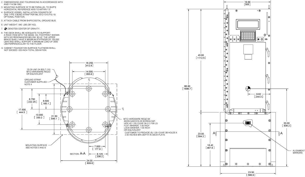
Figure 8-14. Installation Guidance Mounting Arrangement (Sheet 1 of 6)
