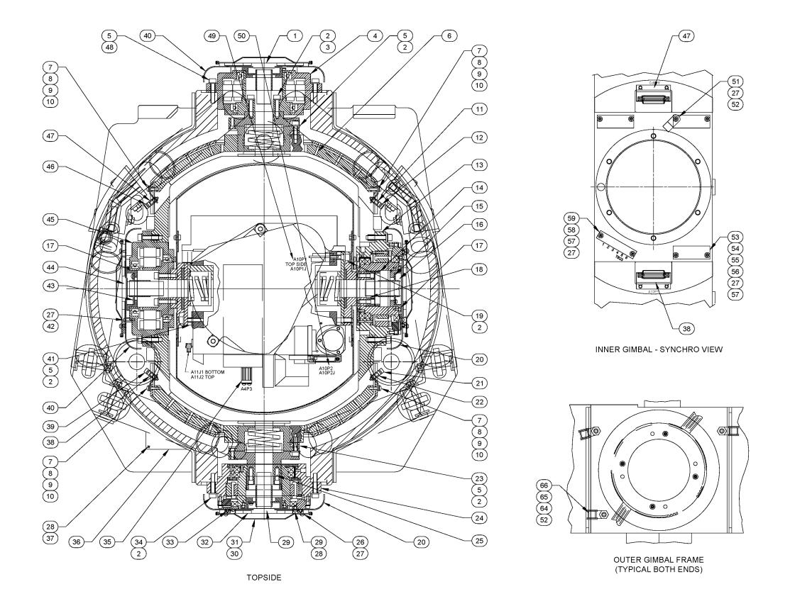
Figure 7-9. IMU: Subassembly Identification (1A2A1A1)
