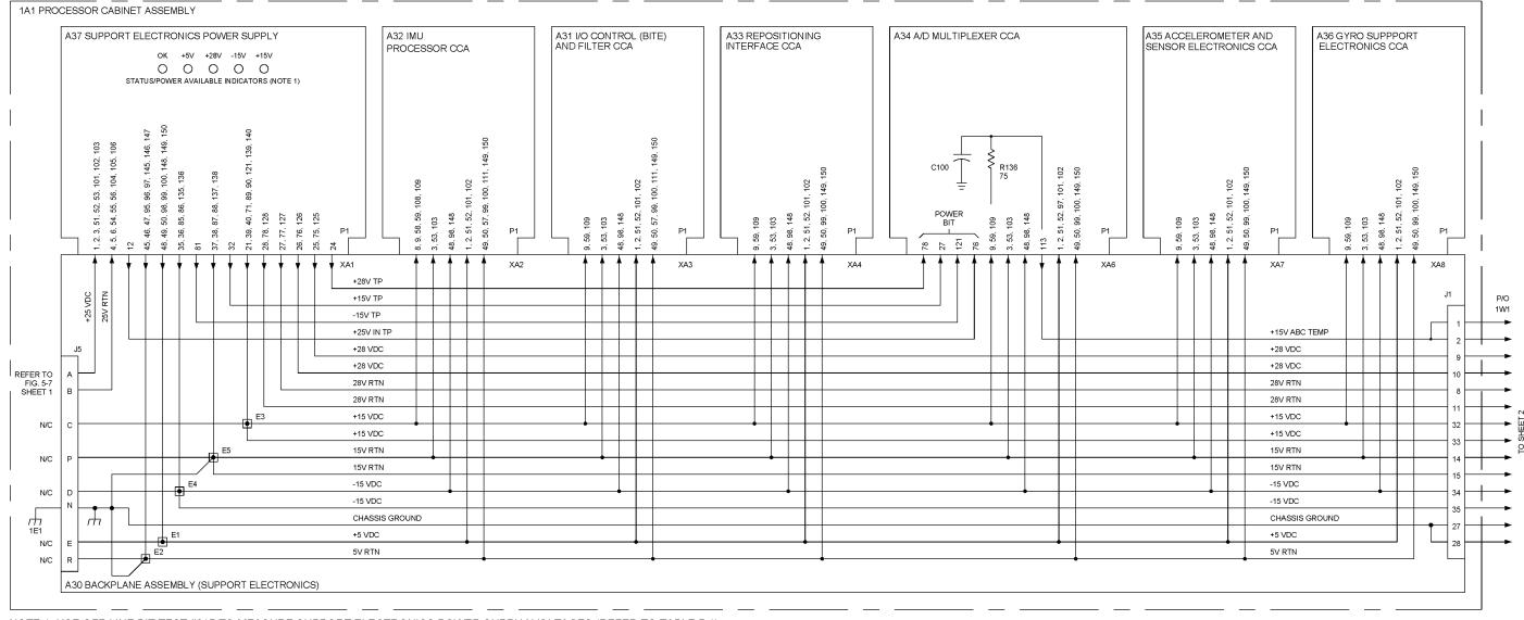
NOTE 1: USE OFF-LINE BIT TEST #315 TO MEASURE SUPPORT ELECTRONICS POWER SUPPLY VOLTAGES (REFER TO TABLE 5-1).
