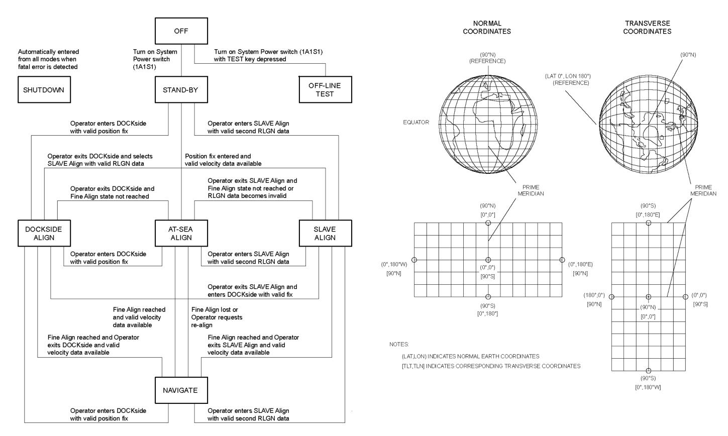
Figure 2-8. Mode Transition Diagram
