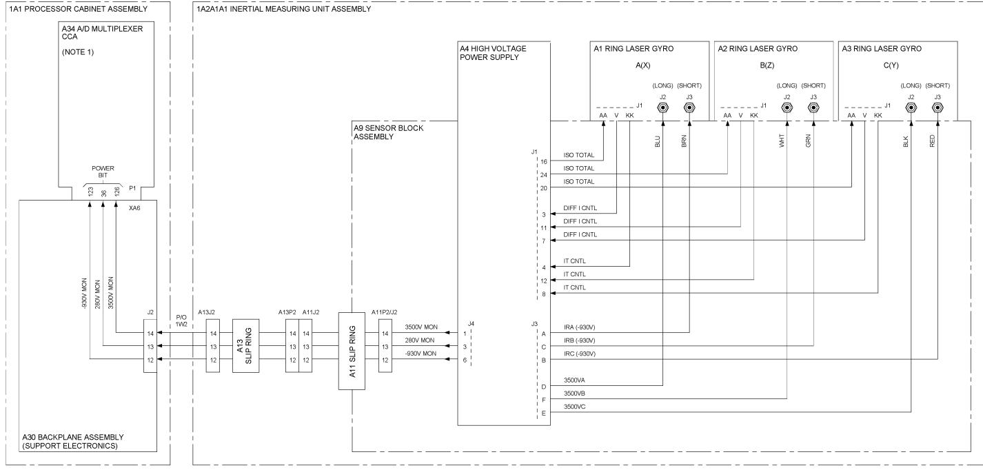
NOTE: 1. USE OFF-LINE BIT TEST #316 TO MEASURE HIGH VOLTAGE POWER SUPPLY VOLTAGES (REFER TO TABLE 5-1).
