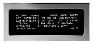
Press the **<SENSOR>** key to access the Sensor menu. Manually select the Navigate mode by selecting **SLAVE OFF** and then selecting a valid velocity-damping source.
