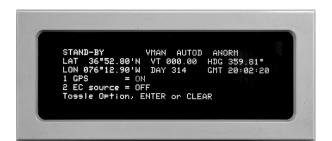
e. Press the **<ENTER>** key. The display will change to show that the GPS has been accepted as a position reference.
