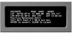
If Vertical Deflection East displays 00.0 arc seconds, press the **<ENTER>** key. If it does not, press the **<CLEAR>** key. Enter +00.0.
