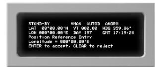
f. Accept or reject the longitude value. If the displayed value is incorrect, enter the ship's longitude within 0.01 nm accuracy. The display shows the ship's fix and prompts the operator to accept or reject the information. STAND-BY VMAN AUTOD ANORM LAT 00°00.00'N VT 000.00 HDG 359.86° LON 000°00.00'E DAY 197 GMT 17:19:58 Fix LAT 36°52.80'N Fix LON 076°12.90'N 17:18:05 ENTER to accept, CLEAR to reject
