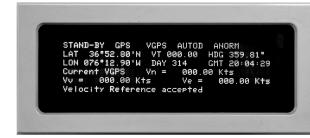
o. The system will automatically sequence to the Navigate mode upon completion of **ALIGN-F**.
