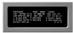
b. Press the <5> key and select RESET DATA. The fix latitude and longitude will be displayed, along with the fix accuracy (FSN and FSE), and the type of fix taken.
