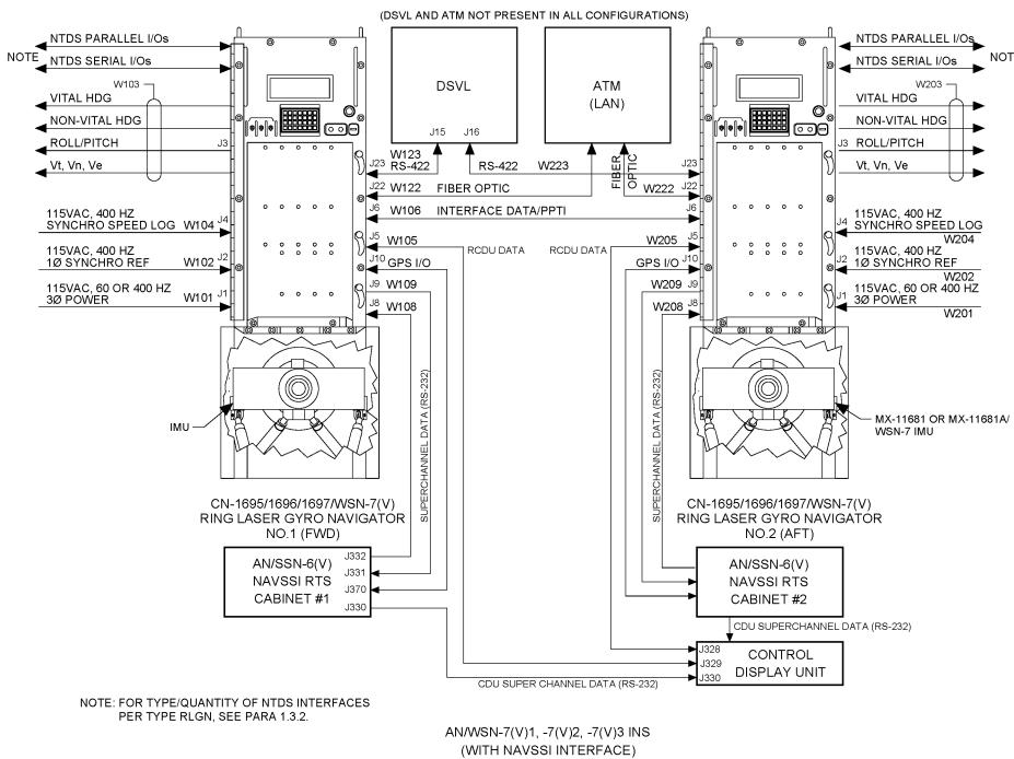
Figure 1-2. Typical System Configuration (Sheet 2 of 2)
