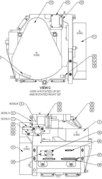
Figure 7-11. IMU: Sensor Block Assembly (1A2A1A1A9)
