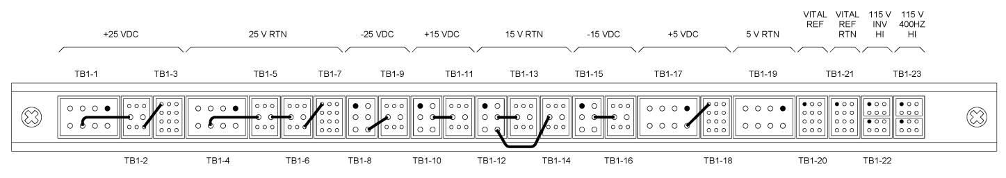
SOLID FILLED PIN INDICATES INPUT CONNECTION FROM POWER SOURCE TO TERMINAL BLOCK GROUP WHICH DISTRIBUTES THE POWER.
