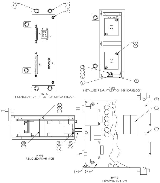
Figure 7-12. High Voltage Power Supply Assembly (1A2A1A1A4)
