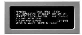
To reject the new position, press the **<CLEAR>** key. To accept the new position, press the **<EN-TER>** key. Observe that Position is accepted.
