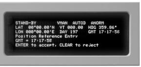
Press the **<ENTER>** key to accept the time or the **<CLEAR>** key to reject and reset the time. The display will show the "Vertical Deflection North" with a value of 00.0 arc sec and prompt the operator to accept or reject it.
