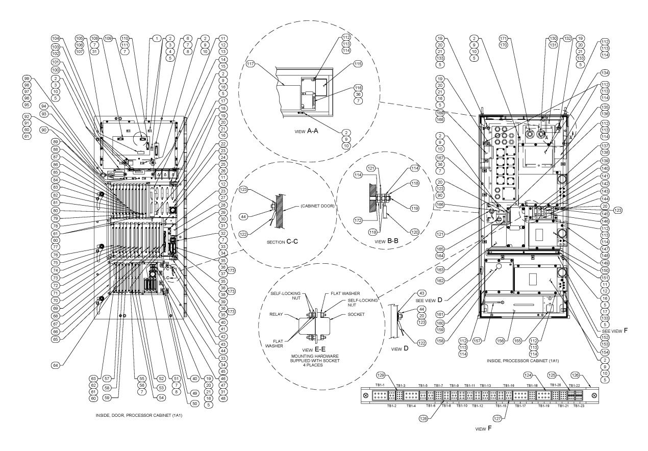
Figure 7-3. Processor Cabinet Assembly (1A1) (Unit 1) Internal Components
