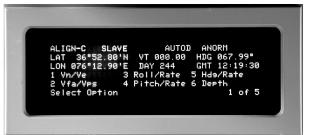
d. Upon completion of Fine Align, verify **ALIGN-F** appears in the upper-left field of the display, indicating completion of Fine Align.
