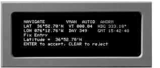
g. To enter a different value, press the **<CLEAR>** key and enter fix latitude in DD°MM.mm' format. Press the **<NE+>** key to enter the North Hemisphere, or the **<SW->** key to enter the South Hemisphere.
