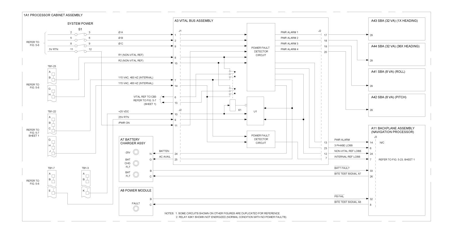
Figure 5-10. Power Fault Detection and Power Control Functions Diagram
