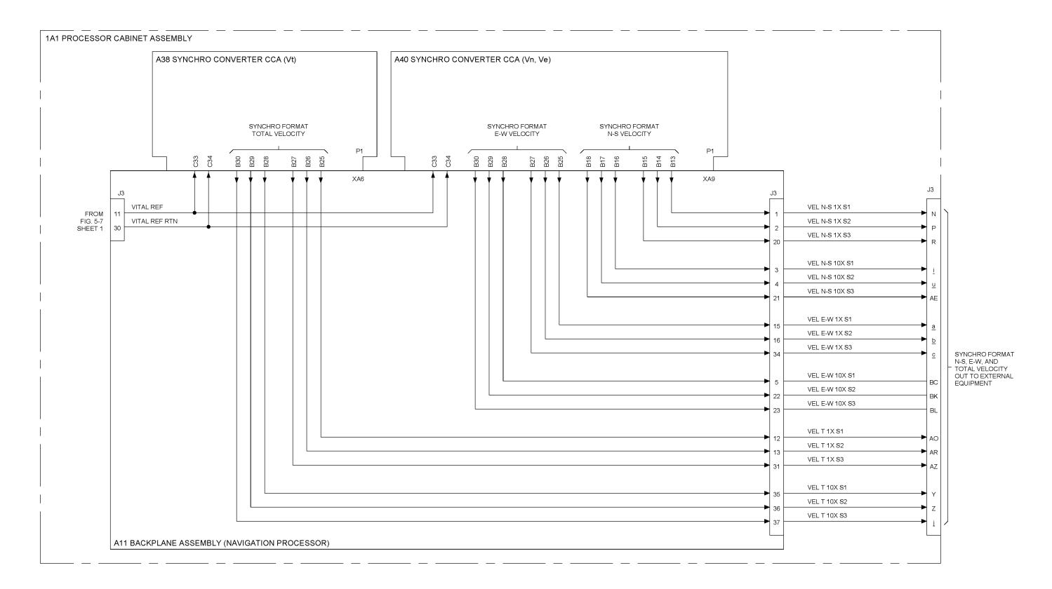
Figure 5-21. System Synchro Format (Heading, Roll, Pitch, and Velocity) Outputs Diagram (Sheet 3 of 3)
