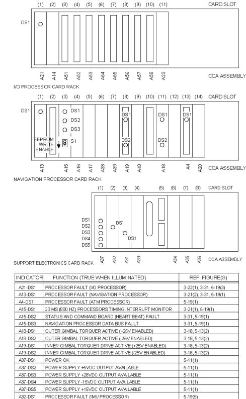
Figure 5-2. Status LEDs and EEPROM Write Enable Switch Identification
