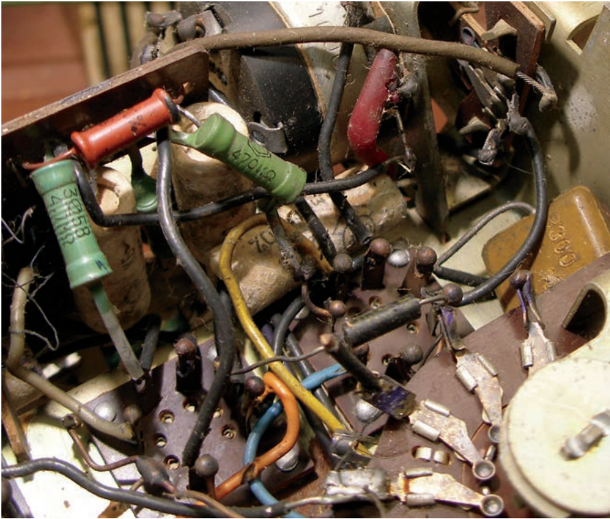
Fig. 14. Note balls of copper formed when prepared mechanical connection is welded. (Author's collection)
