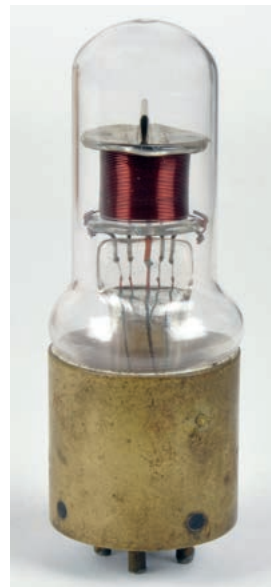
Fig. 9. An early prototype Solenoid tube used to test a concept for supporting the solenoid spool by using the glass envelope. (Lauren Peckham Collection)
