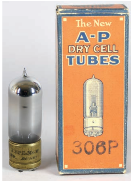
Fig. 23. Evidence that A-P Radio Laboratories made a Type 306M with a UV base in addition to a Type 306P tube, both of which were characterized as a “peanut tube.” (Joe Knight Collection)
