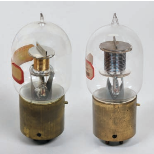
Fig. 8. Two of 38 Solenoid tubes made in 1923, which were used in an extensive test program to determine the optimum design parameters for a production tube.
