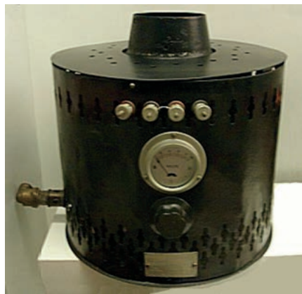
Fig. 1. Thermattaix gas powered generator for charging filament batteries. (Science Museum, London)
