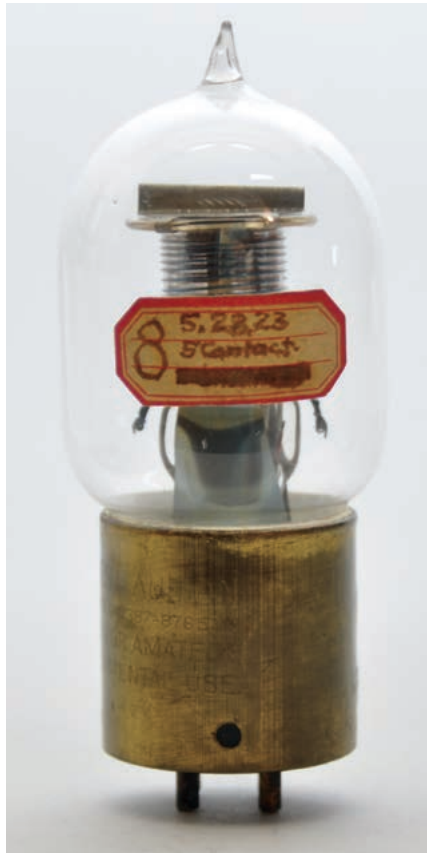
Fig. 11. One of 38 prototype vacuum tubes made in 1923, each of which had a white sticker with a red border affixed to the glass bearing a number in the order of testing (8), the date it was tested (5.28.23), and a key descriptor (5 contact). (Huppert papers)
