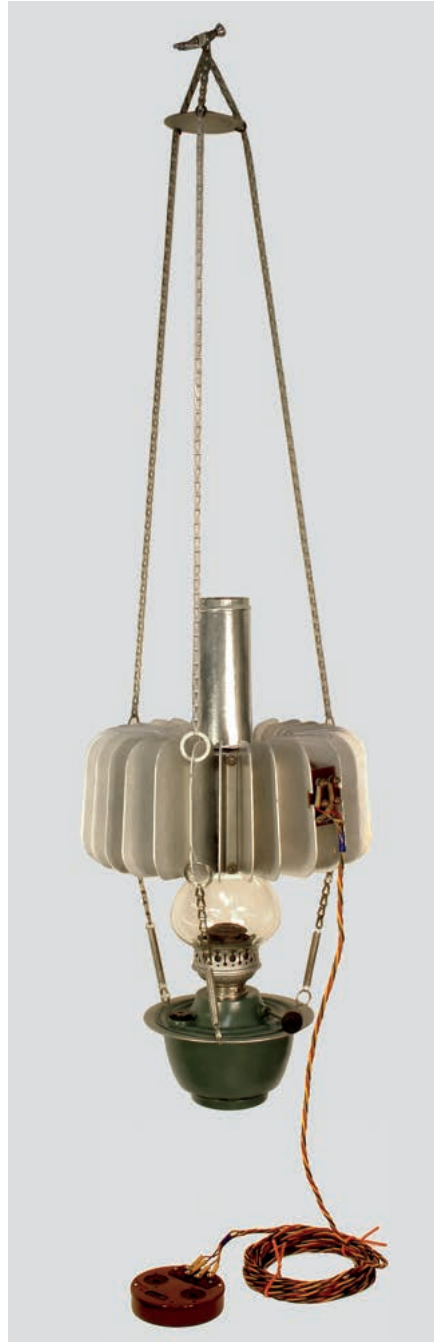
Fig. 5. A TZGK-2-2 (1958) Thermoelectric Generator. (Author's collection)
