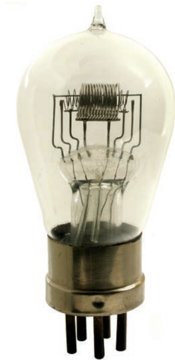
Fig. 27. The four-electrode K4 tube introduced by the Bower Electric Company of England earlier in 1924 under the Thorpe trade name. (The National Valve Museum)
