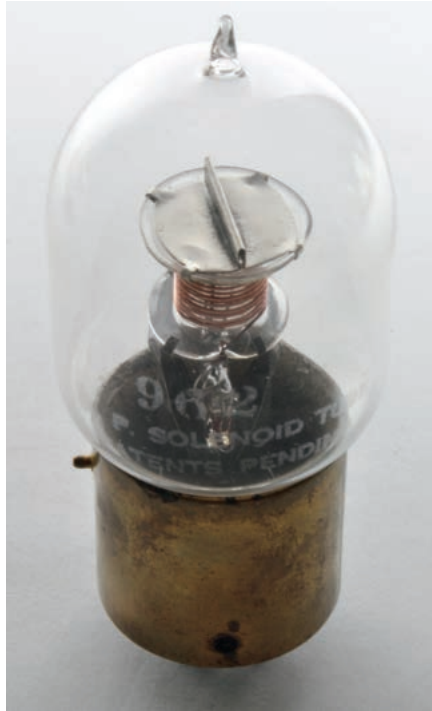
Fig. 13. A production Solenoid tube stamped with the number 962 followed by "A. P. Solenoid" and "Patent Pending."
