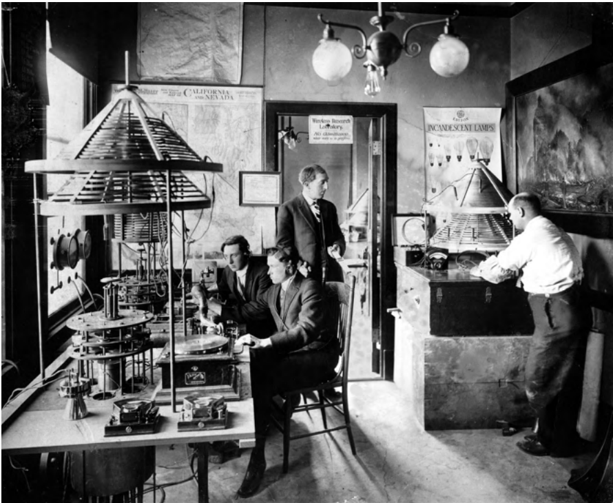
Fig. 3. This famous scene of Charles Herrold in his makeshift “broadcast studio” was posed in 1912 with his so-called “arc fone” transmitter. A water-cooled carbon telephone used as a microphone can be seen right next to a small horn on the phonograph. (Author’s collection)
