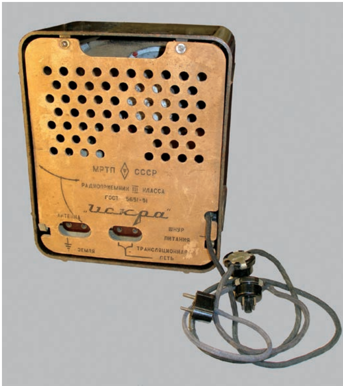
Fig. 17. Back panel of Spark (1958) showing connection for "cable radio" input. (Author's collection)
