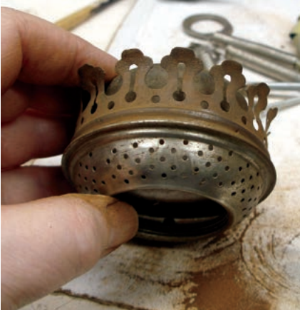
Fig. 8. Burner made of four swaged stampings, some too rusted to be re-plated. (Author's collection)
