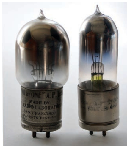
Fig. 22. The 625A and 625D with 6-volt filaments had a Shaw base with a classic Moorhead glass envelope (left), but the 306A with 3-volt filaments had a tubular shaped glass envelope (right).
