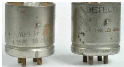
Fig. 20. The Type 625A Two-in-One nickel tube base is stamped with “Amplifier” (left), and the Type 625D nickel tube base is stamped with “Detector” (right).
