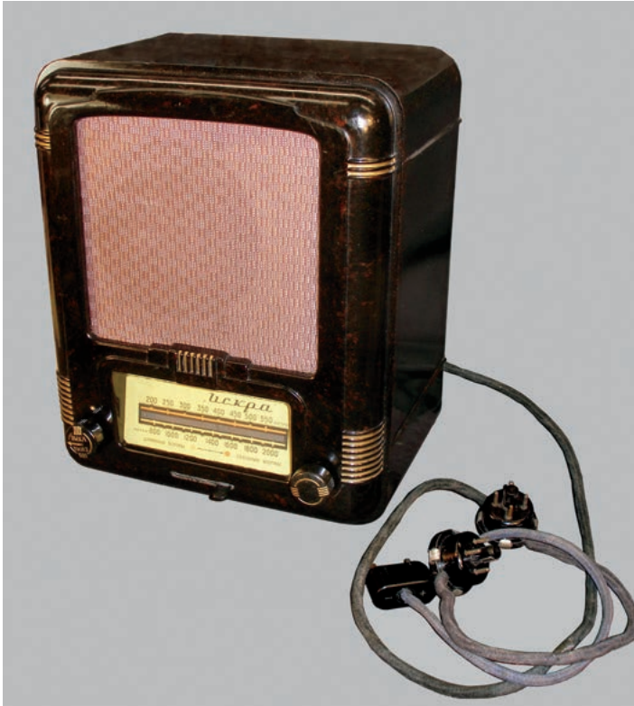
Fig. 10. This Spark battery-powered receiver was made in 1958. Note plugs for connection to standard batteries. (Author's collection)
