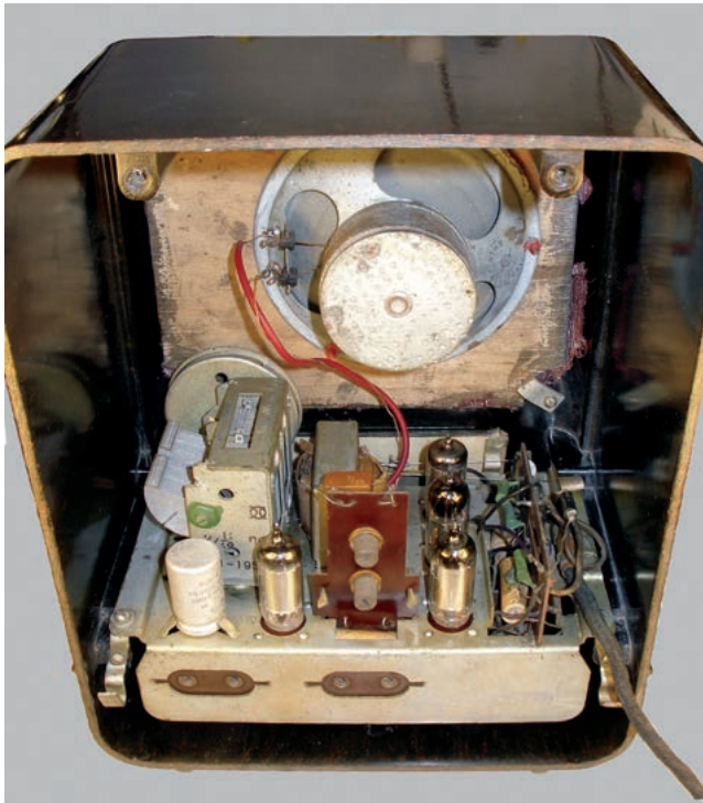
Fig. 13. Back cover removed on 1958 version of Spark receiver. (Author's collection)
