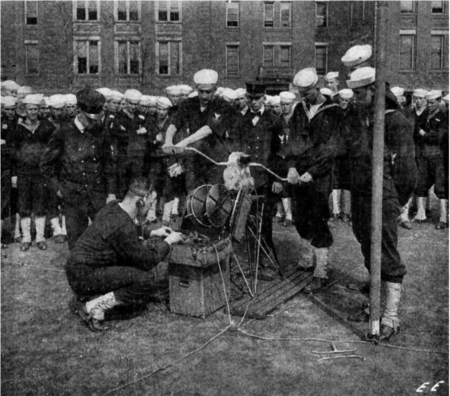
Fig. 28. Outdoor demonstration of portable radio equipment, a suitcase pack set, and a hand generator at Harvard. ( Electrical Experimenter , Dec. 1918, p. 548)
