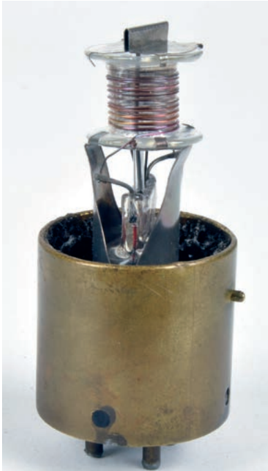
Fig. 12. A close up photograph of a tube without its glass envelope, believed to be a production tube based on the prototype No. 16. (Loren Peckham Collection)
