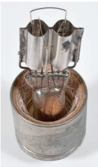
Fig. 19. A photograph of the interior of a Two-in-One tube that is missing the glass envelope.
