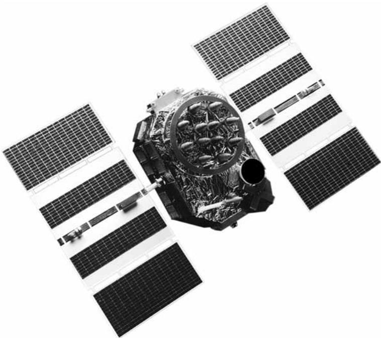
**Figure 3.6** Block IIA satellite.
