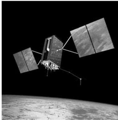
**Figure 1.2** GPS III satellite. (Courtesy of Lockheed-Martin.)
