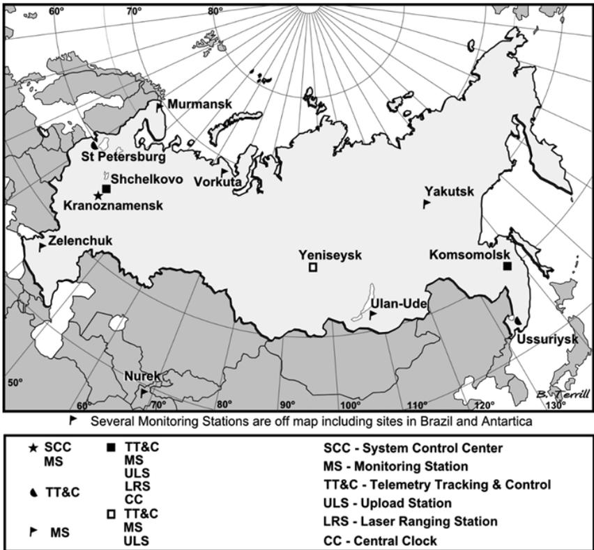
Figure 4.7 GLONASS ground segment.
