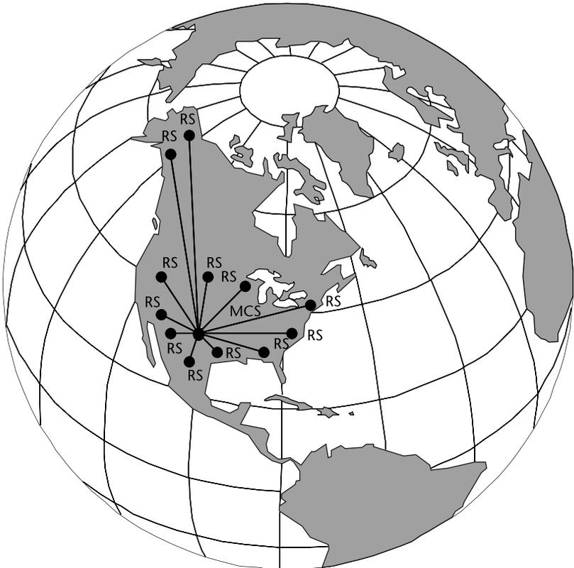
Figure 12.3 WADGNSS concept.
