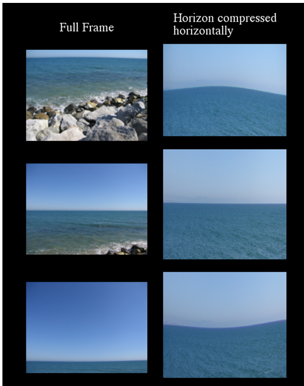
Fig. 4. (Color online) Apparent curvature of the horizon. On the left, the full frames are shown. On the right are the horizon photos cropped and compressed 10 : 1 horizontally to enhance the barrel distortion.
