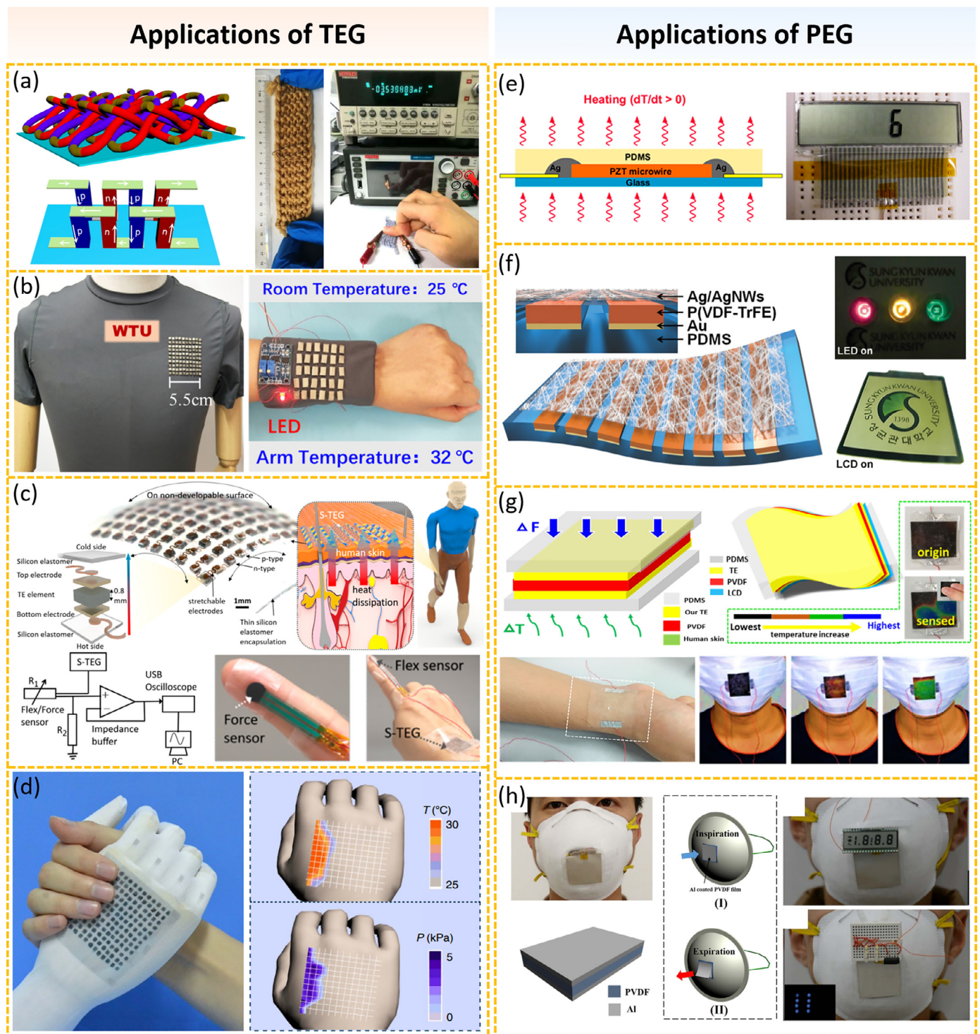
Fig. 3. Applications of thermal energy harvesting technology. (a) A stretchable all-fabric TEG based on woven thermoelectric fibers. (b) Thermoelectric units array integrated with a T-shirt and a wrist strap. (c) A stretchable and shape-adaptive TEG integrated with a force sensor. (d) A self-powered temperature–pressure dual-parameter sensor array based on microstructure-frame-supported organic thermoelectric materials. (e) A PyNG consisting of a single lead zirconate titanate microwire. (f) A highly stretchable PyNG based on micropatterned architectures. (g) A flexible transparent tribo-piezo-pyroelectric hybrid generator for physiological monitoring. (h) A self-powered breathing sensor based on a PVDF film integrated with a mask.
