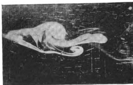
FIG. 20.—The Eddies of Fig. 19 have Expanded and Been Torn Away. The Direction of Stream Lines is Shown by the Short Bright Streaks.
