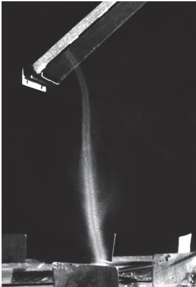
Figure 5.4. Compression of a gas vortex at the air intake of an airplane jet engine (at parking)
