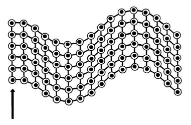
Fig. 6. A plane lattice transmitting shear waves.
