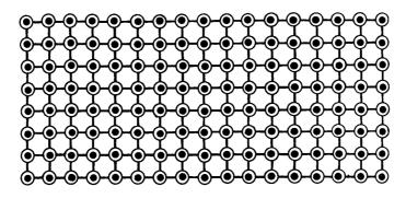
Fig. 5. A plane lattice consisting of unit masses, rigid links and hinges.
