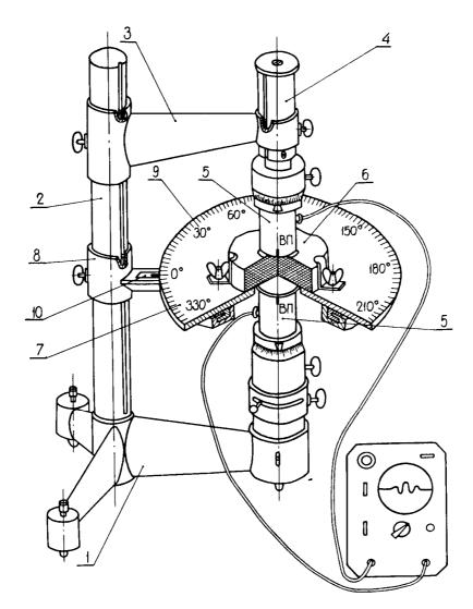
Fig. 1. Design of acoustopolariscope with the rotating platform (Pat. No. 1281993, USSR). 1 - base; 2 - pole; 3 - bracket; 4 - travelling rod; 5 - transducers; 6 - sample; 7 - rotating platform; 8 - additional bracket; 9 - angle scale; 10 - mark.
