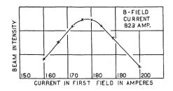
FIG. 6. Intensity of beam against field with selector slit interposed to pass only atoms with negative moments, for hydrogen.
