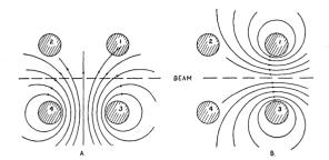
FIG. 2. Diagrams of field near wires T. (A) Nonadiabatic field; (B) Adiabatic field.
