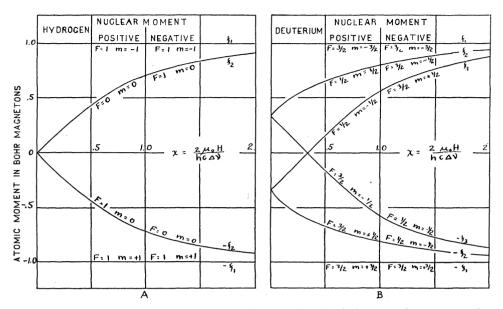
FIGS. 1A and 1B. Diagram to show quantum numbers associated with the magnetic states assuming the nuclear spin positive or negative.
