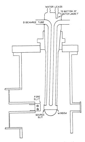
FIG. 4. Section of source chamber to show the construction of discharge tube and of the eccentric brass adjusting collar.
