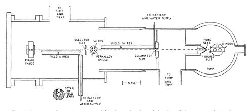
FIG. 3. Diagram of apparatus as used for determination of the sign of the moment for hydrogen and deuterium. The permalloy shield and the wires T were removed from the apparatus for the measurement of the magnitudes of the moments.
