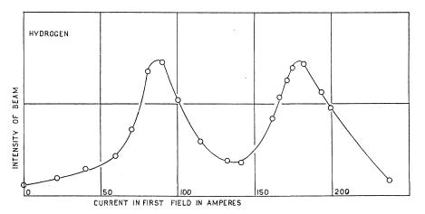
FIG. 5. Intensity at center of beam against field current for hydrogen to show nuclear spin to be  $\frac{1}{2}$ . The first peak is for  $\pm f_1$ ; the second for  $\pm f_2$ .
