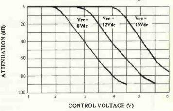
Fig. 3. Attenuation characteristic of Motorola MC3340
