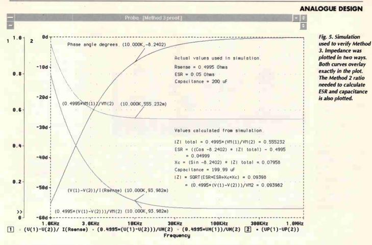
Measured voltage and phase angle agreed closely with the simulation. The ESR and capacitance values obtained from my measurements were within 5% of the capacitance and ESR for the assembly, Fig. 4.
