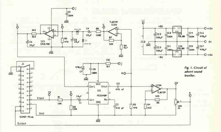
When the sound becomes louder, voltage at D increases. increasing the attenuation. Thus the sound level at B remains constant.
