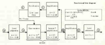
Fig. 2. Block diagram of advert sound leveller.
