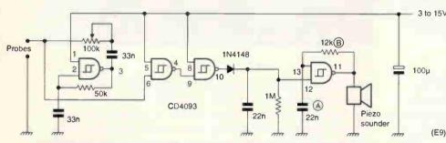
Low cost, long battery life and adjustable sensitivity are features of this liquid level sensor circuit. If you want a logic-level output, tie pin 13 to  $V_{cc}$  and omit components A and B.
