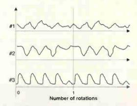
Fig. 1. Notional variation of sensor parameter as a function of degree of rotation and with the cycle repeating itself every revolution.
