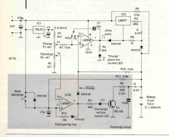
With experience, the flash rate of the green LED can indicate the state of charge of the battery. With new and fully charged batteries, the period between flashes is several seconds. Use of high current pulses up to C avoids the memory effect in NiCd cells.
