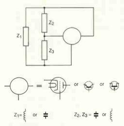
Fig. 2. Varieties of Fig. 1a) type oscillator based on a maintaining amplifier. No separate feedback winding is involved here.
