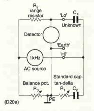
Fig. 1. Showing the basic bridge circuit for capacitance measurements.
