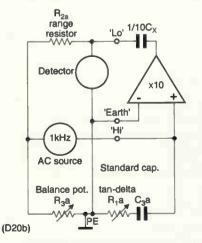
Fig. 2. Outline arrangement to extend the smallest range from 100pF maximum to 10pF maximum.
