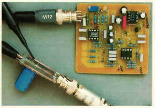
Fig. 3. Using test jig 2, Method 2, to measure impedance, with a high input-impedance meter. My stack of three 1218 surface mount chip resistors, total resistance 0.4989 $\Omega$ , are visible near the test-probe ground clip. Compared with Fig. 1, the test voltages, VM(1) and VM(2) have larger magnitudes. This facilitates both voltage and phase measurement.
