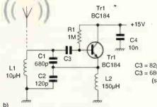
Thus the received signal is demodulated and available at the collector of  $Tr_1$  – you have a simple 'super-regen' receiver.
