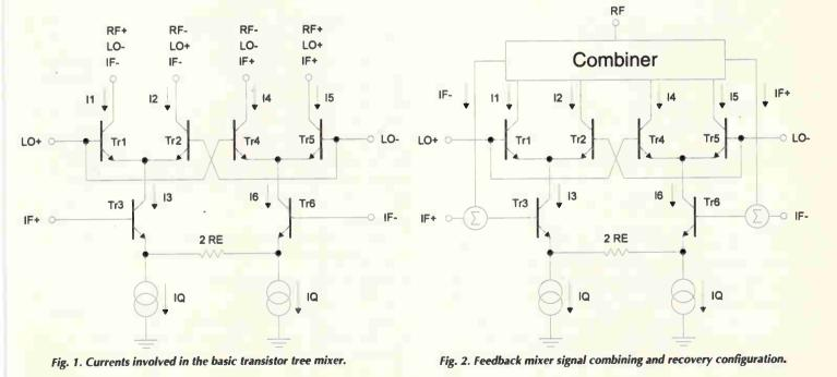
a guide. In a general sense, the desired outcome of the mixer is to have an output RF signal that is a linear combination of the input intermediate-frequency and local-oscillator signals.
