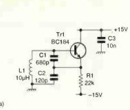
the transistor begins to conduct, the RF oscillation rapidly builds up again, resulting in the next cycle of the squeg frequency - a much lower frequency than the r.f. oscillation frequency.
