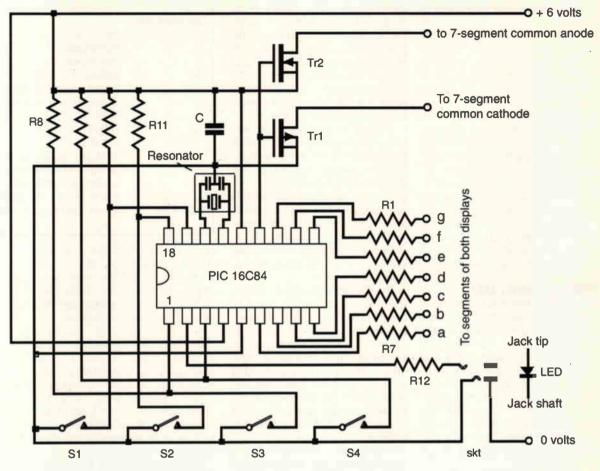
Fig. 1. Complete circuit of the flicker fusion meter, apart from the display. All 13 i/o lines of the PIC16C84 are used. The controller can be set to work with a crystal, resonator or RC network, depending on the accuracy you need. In this application, a ceramic resonator is the best compromise. been designed to measure CFF in the workplace<sup>6</sup>.
