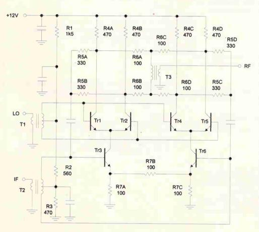
the CA3054 for the transistor array using the components values shown in Fig. 3. For  $T_1$ ,  $T_2$ , and  $T_3$ , we used the Mini-Circuits T4-1 transformer.
