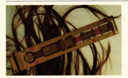
Hairing aid... Micro-via PCB technology called DYCOstrate has been used to implement a programmable hearing aid by Swiss firm Sulzer Microelectronics. This hearing aid is the smallest of its type, the firm claims. The extreme packaging needs of a hearing aid led the firm to use the flexible substrate which can be folded up after manufacture. DYCOstrate is available in the UK through Rigid and Flex.
