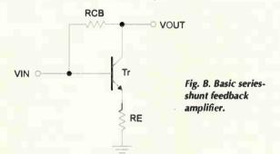
This circuit, shown in Fig. B, is a good example of how the simplest of inventions can be the most profound. These simple wide-band amplifiers are easily designed using the following simple relationships for input/output resistance and gain:
