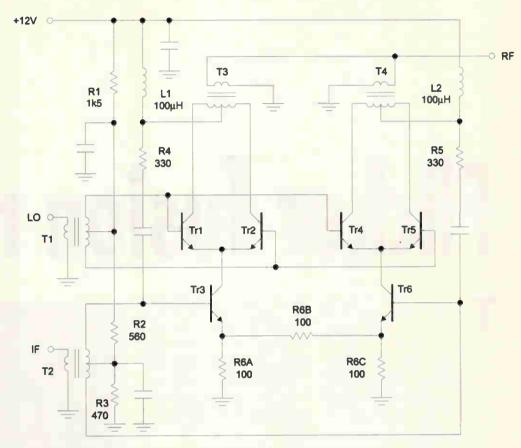
Fig. 4. Second-generation series-shunt feedback mixer. Adding a pair of hybrid transformers to combine the four collector currents eliminates the compromises of this circuit's predecessor.
