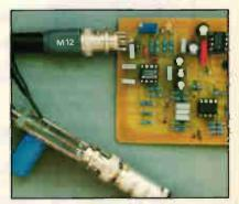
To evaluate a capacitor for a modern switched-mode power supply, a good test jig is vital. Find out what Cyril Bateman uses on page 696.
