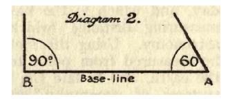
Now if we know the length of the base-line A B, in feet, yards, kilometres or miles, (to be ascertained by actual measurement), and also know the value of the two angles which indicate the direction of a distant object as seen from A. and B., we can readily complete the triangle and so find the length of its sides. In this way we can measure the height of a tree or church steeple from the ground level, or find the distance to a ship or lighthouse from the shore.
