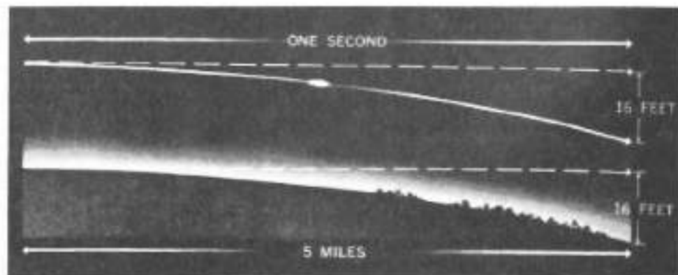
Figure 1: At five miles per second, a near-earth satellite falls toward earth at the same rate as the earth's surface curves underneath it. Thus the satellite stays at the same height above the surface of the earth and remains in orbit.
