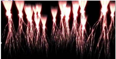
Below: Lichtenberg figures as created from high-energy dielectric saturation into Lucite, then discharged along a grounded spike
