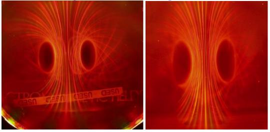
**Below:** [Photo courtesy of Michael Snyder of revolution-labs.com] Broken ring magnet illustrated by the Timm Vanderelli ferrocell. Notice the color displacements. The red exists along the center where there is lower dielectric voidance, and the yellow exists along the interior rim as does the green.
