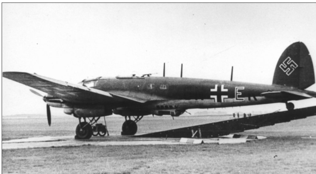
Heinkel 111 of Kampfgruppe 100 on the compass swinging base. Note the two additional aerial masts on the rear fuselage, belonging to the X-Gerät beam attack system.
