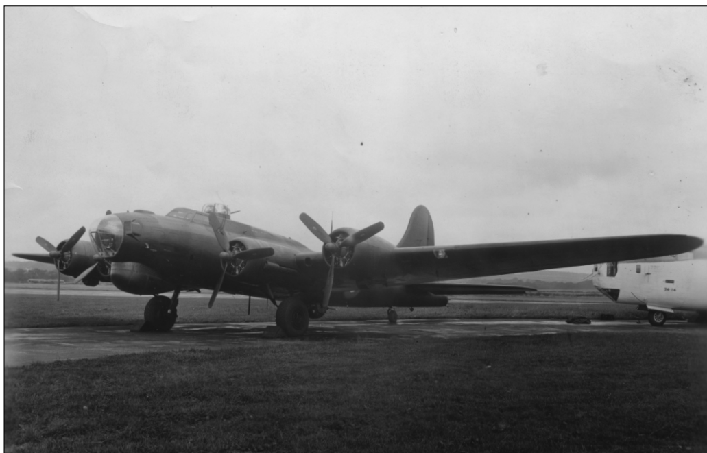
B-17 Flying Fortress modified as a jamming escort aircraft, before issue to No. 214 Squadron, RAF. The radome under the nose housed the scanner for the H2S radar.
