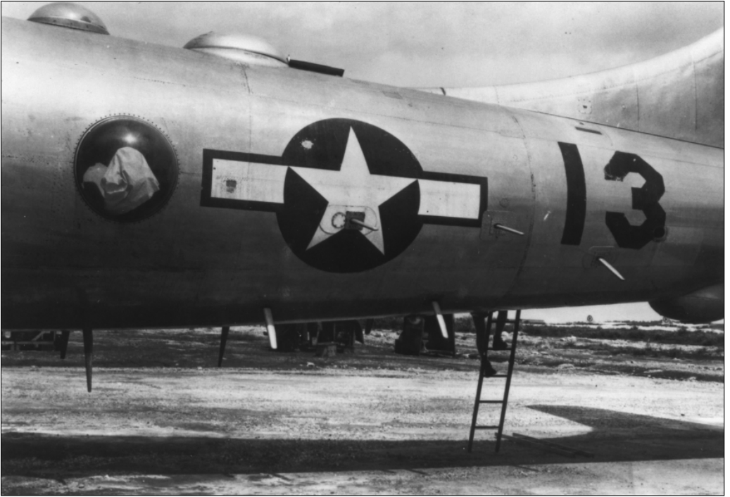
'Guardian Angel' B-29, which served as a jamming escort aircraft to provide cover for bombers attacking Japan. Eight jamming aerials are visible on this view of the aircraft.
