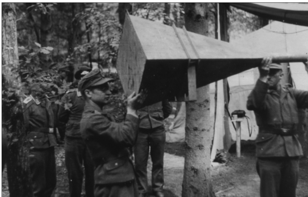
Aerial of a Korfu ground direction-finding station, which tracked RAF bombers by picking up the radiations from H 2 S.
