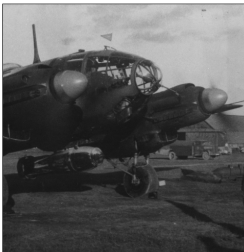
Heinkel 111 bomber of III/KG 26, the unit which employed the T-Gerät beam system over Britain in 1940–41. Note the additional aerial for the system, mounted above the fuselage behind the cabin.
