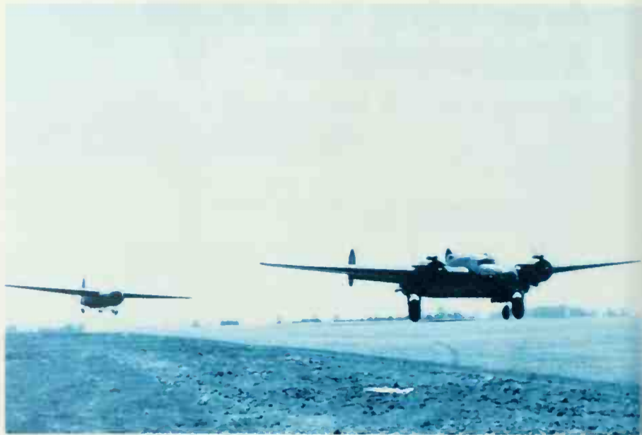
Above: An Albemarle, probably an ST.II, on takeoff with Horsa I at the Heavy Glider Conversion Unit, Brize Norton.
