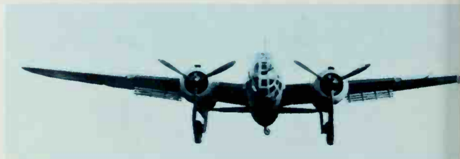
Above: The Ki-48-IIb was fitted with snow-fence type dive-bombing airbrakes above and below the wings.
