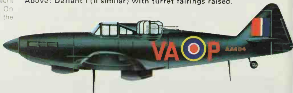
Above: Defiant I (II similar) with turret fairings raised.
