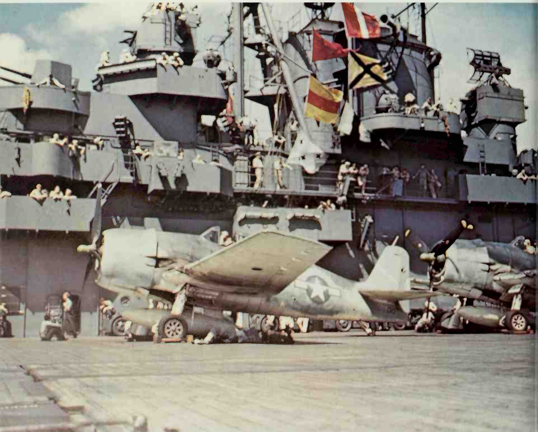
Below: F6F-3 Hellcat pilots waiting to start their engines for a mission, aboard a US Navy carrier in the Pacific. The F6F-5 differed in having extra armour, better cowling and other details.
