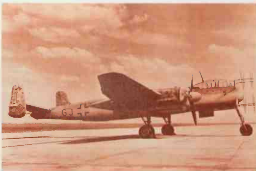
The He 219A-7/R4 had exceptional high-altitude equipment and performance, plus ejection seats, but armament was reduced to four MG 151/20, all firing ahead. This was relatively light.
