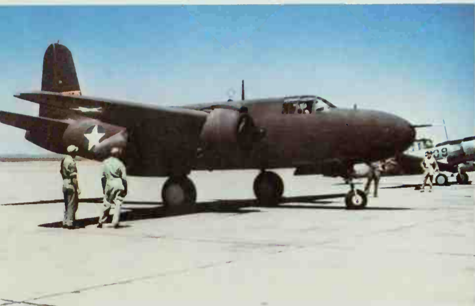
Above: There were many intruder sub-types. This is an early P-70A with the nose armament later fitted to some A-20G attack bombers: four 20mm M-2 cannon. This example has no radar.
