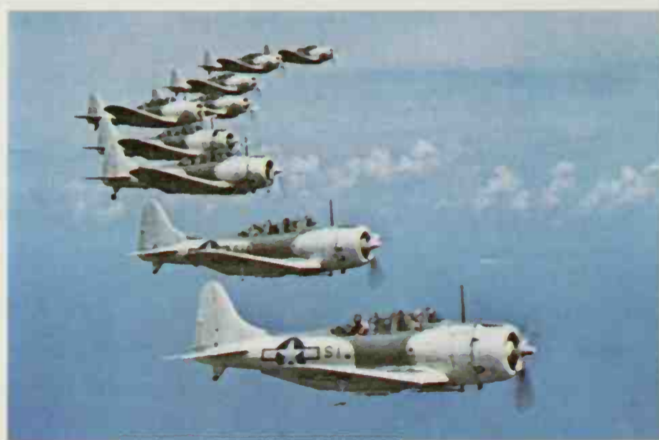
Above: This squadron probably has the SBD-5 or -6, but differences between sub-types were mainly internal. ASV radar was introduced with the -4, together with radio nav aids.
