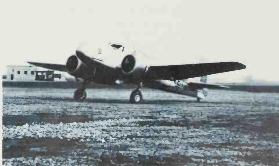
Above: The Ca 310 Libeccio was the first of the family to have retractable landing gear. Later versions were more powerful.
