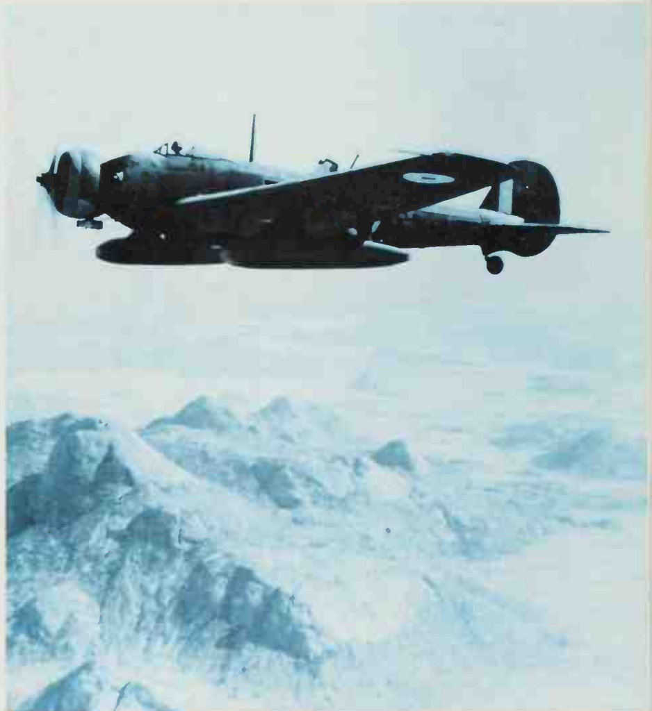
Above: The Wellesley saw most of its service in east and north-east Africa in 1940-42. This example, pictured in 1940, has the hood of the rear cockpit swung open and the gun ready for action. The containers housed the bombs.
