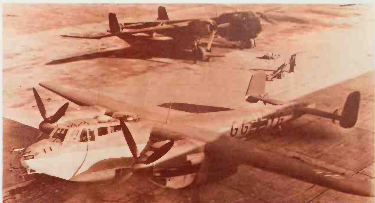
Above: First flown on 31 July 1942, the DB-powered Do 217N-1 night fighter reached NJG units before the end of the year. The FuG 202 Lichtenstein BC radar aerial is prominent; the N-2 dispensed with the turret. Behind is an experimental E.
