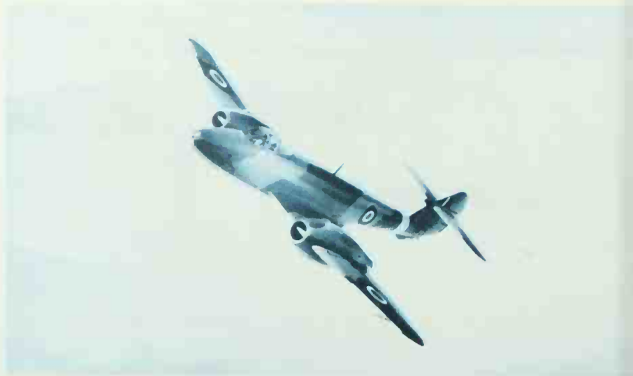
Above: The sliding canopy identifies this as a Meteor III, in service with 2nd TAF squadrons in early 1945. From the 15th Mk III the engine switched to the new Derwent.
