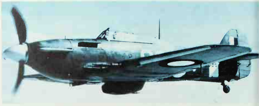
Above: Seen in post-war markings, this Hurricane (Langley-built IIC BD867) shows the constant-speed propeller that became standard in 1941.
