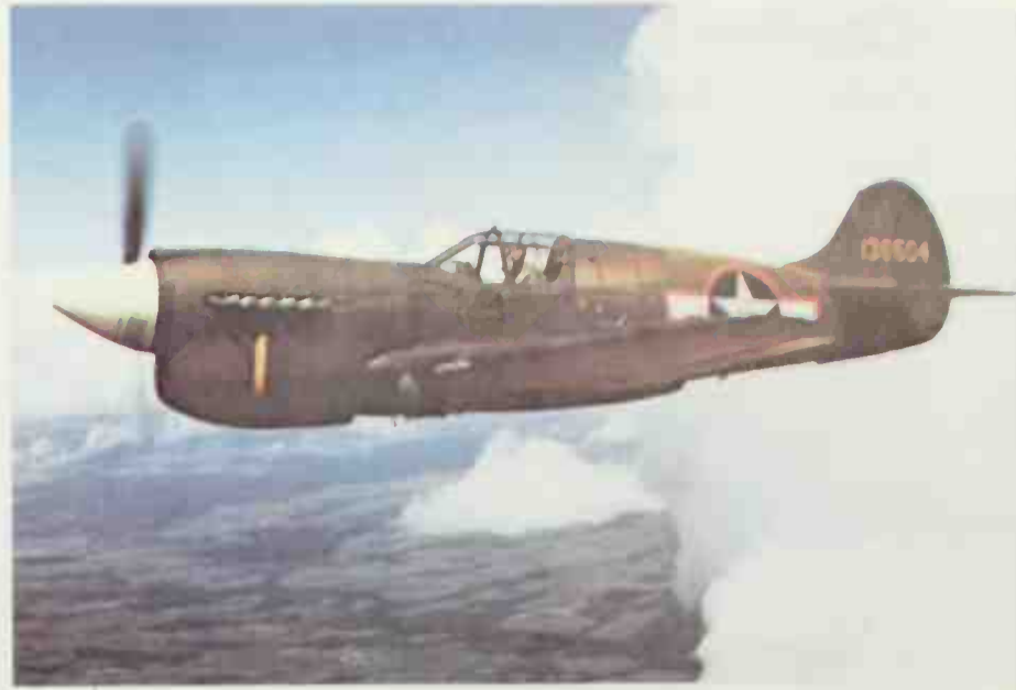
Above: Air-to-air of a middle-vintage P-40E (modified to K standard with anti-swing dorsal fin) with the definitive armament of "six fifties", two more than on the D. The red-outlined insignia soon gave way to dark blue.
