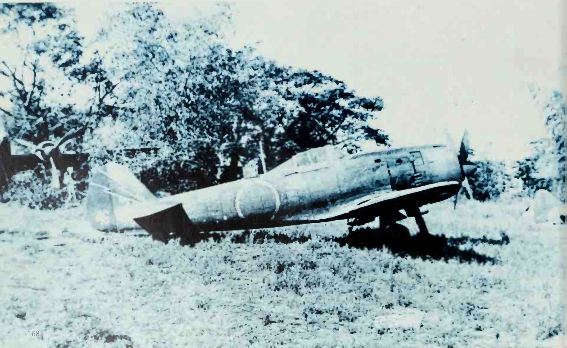
Below: Yet another of the early Ki-84-la models, in this case belonging to the 11th Sentai in the south-west Pacific in mid-1944. Just beneath the trailing edge of the wing can be seen the combat manoeuvre flaps in the 'down' position.
