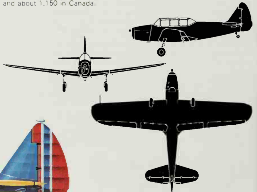
Above: Three-view of PT-26 with in-line engine and enclosed cockpits.
