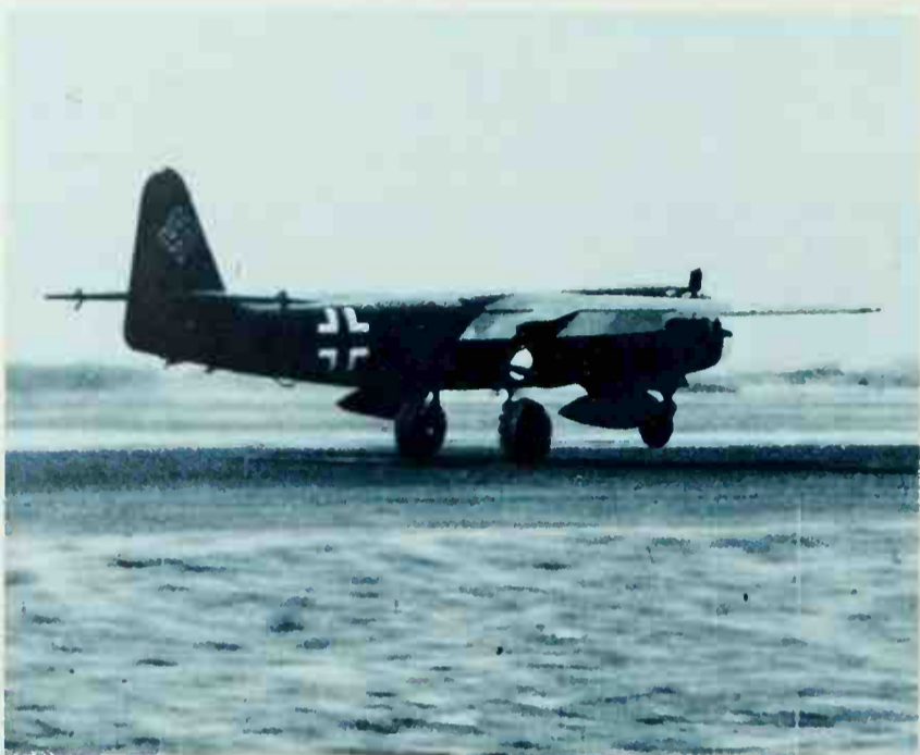
Above: Take-off by the Ar 234 V9 (ninth prototype), first of the B-series with conventional landing gear. Other advanced features included pressure cabin, ejection seat and computer.
