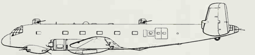
Above: The Ju 188C, with hydraulic tail barquette (abandoned).
