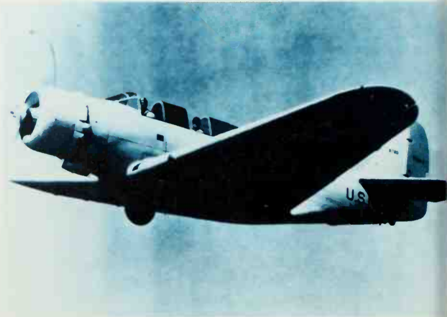
Above: In its day the TBD was an excellent aircraft, but that day was drawing swiftly to a close when the US Navy found itself at war on 7 December 1941. Its wing area was by then appropriate to aircraft of twice the weight and three times the power of the very early-series Twin Wasp engine.
