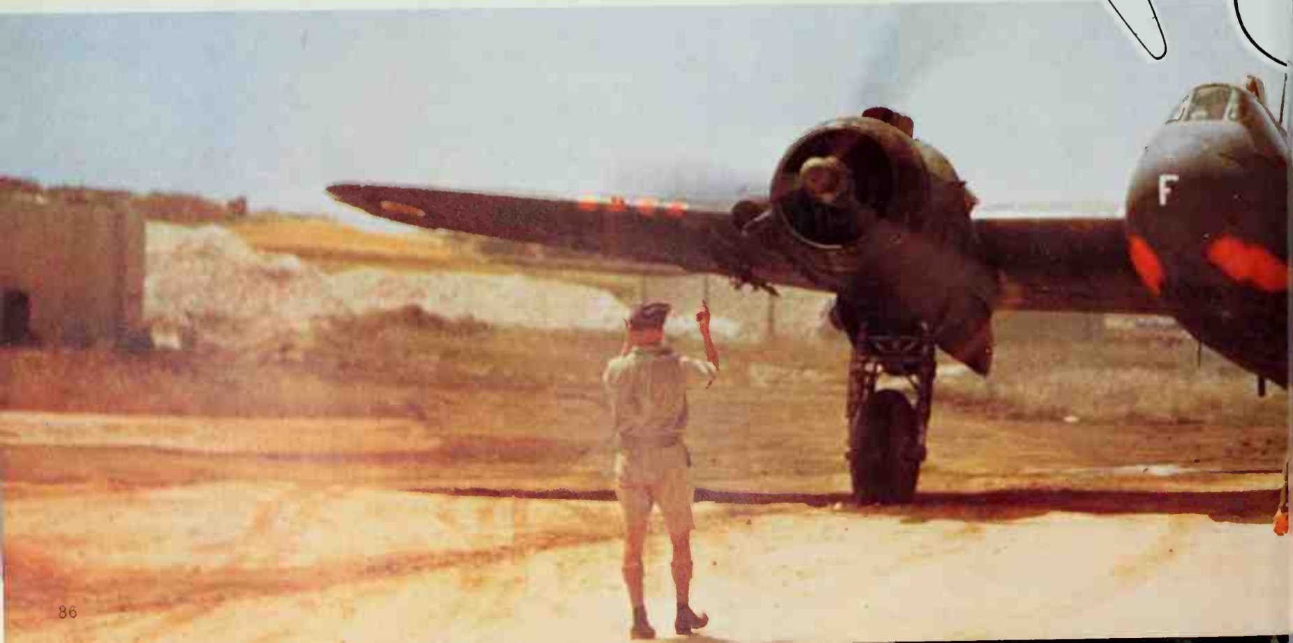
Below: Tough defender of Malta, this Mk IF has underwing bomb racks. Red-doped fabric covers the muzzles of the guns.
