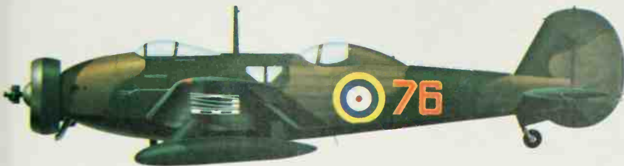
Above: The Wellesley saw most of its service in east and north-east Africa in 1940-42. This example, pictured in 1940, has the hood of the rear cockpit swung open and the gun ready for action. The containers housed the bombs.
