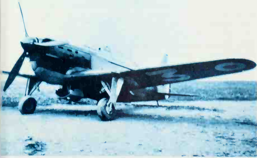
Above: An M.S.406C-1 with the coolant radiator wound down to the fullest extent. In the air the radiator was progressively cranked up into the fuselage to try to reduce aircraft drag, but the long ventral radio aerial was extended.
