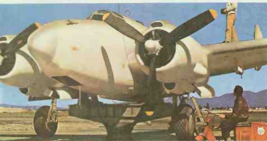
Left: Swinging the compass of a white PV-1 of the US Navy. Many of these multi-role aircraft carried Mk IV ASV radar.
