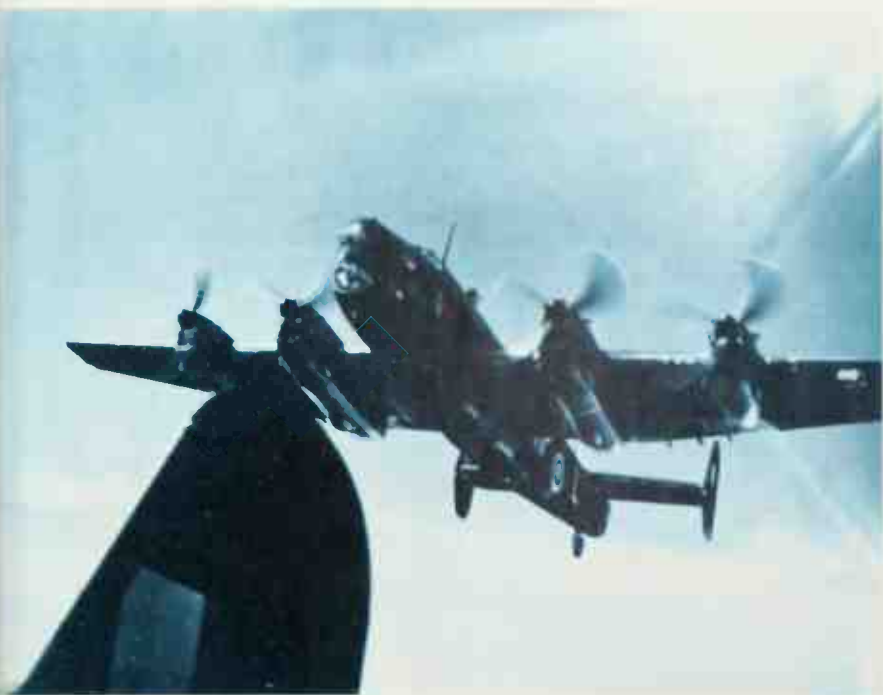
Above: L9530 was one of the first production batch in 1940. Serving with 76 Sqn (MP-L) it had manual beam guns and prominent fuel-jettison pipes passing beneath the flaps. The photograph must have been taken from the right beam gun position of an accompanying Halifax, in mid-1941.
