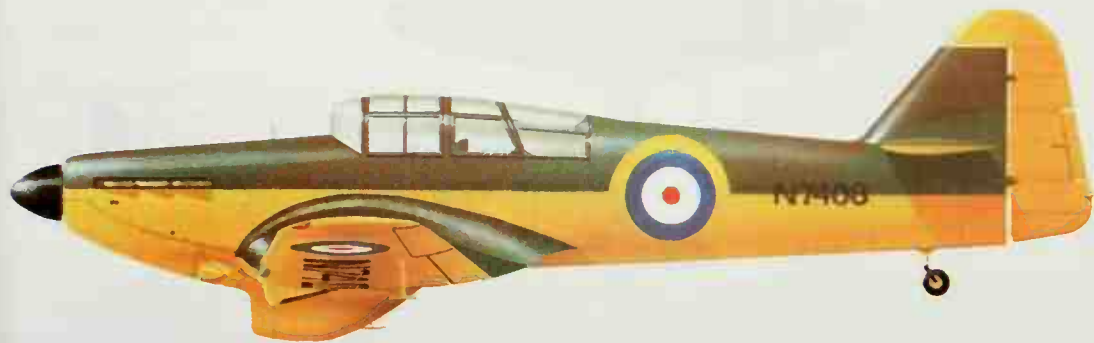
Left: N7408 was the first production Master I. Later the canopy was made taller, with framed, inclined windscreen.
