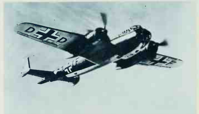
Above: The sixth pre-production Do 217E-0 was used by BMW for engine development.
