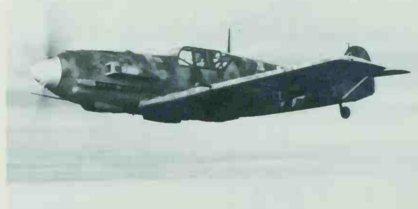
Above: One of the last Bf 109E sub-types, this is an E-7, seen with a large dust filter on the engine air inlet. It was operating on the Leningrad front in 1942 with JG 5.
