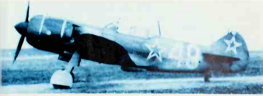
Above: The La-7 had the same engine as the La-5FN but a considerably superior performance was gained by aerodynamic refinement. Total production of all Lavochkin 5/7/9/11 neared 37,000.
