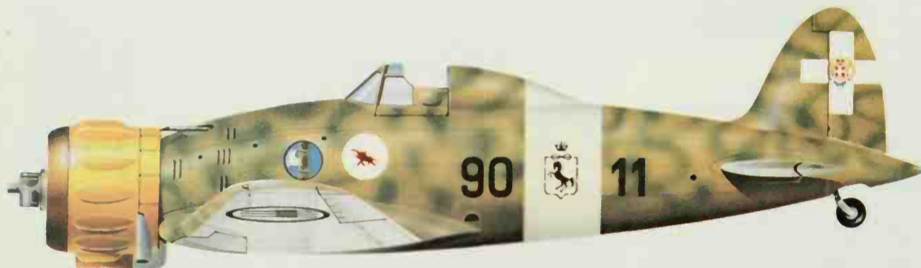
Left: A Macchi C.200 (or M.C.200 for Mario Castoldi) of a late serie in which the original sliding canopy had been replaced by a hinged hood open at the top. This one served the 90o Squadriglia, 10o Gruppo, 4o Stormo, based in Sicily in 1941.
