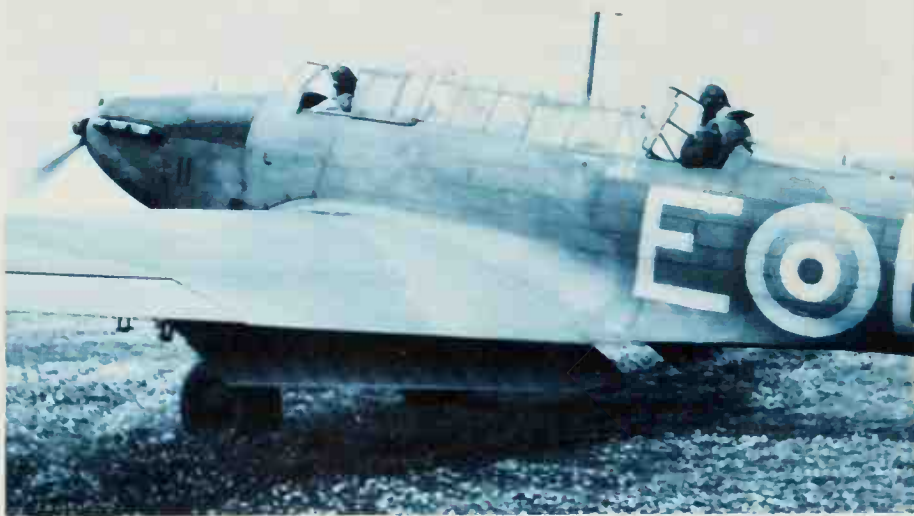
Above: Flap position suggests this Battle has just landed. The yellow roundel ring was added to most Battles after the débacle in France, where the usual roundel was equal radii red, white and blue, often with striped rudder (not fin).
