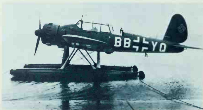
Above: Built in small numbers in 1941, the Ar 196A-4 served on catapults of Kriegsmarine warships and preceded the A-3.
