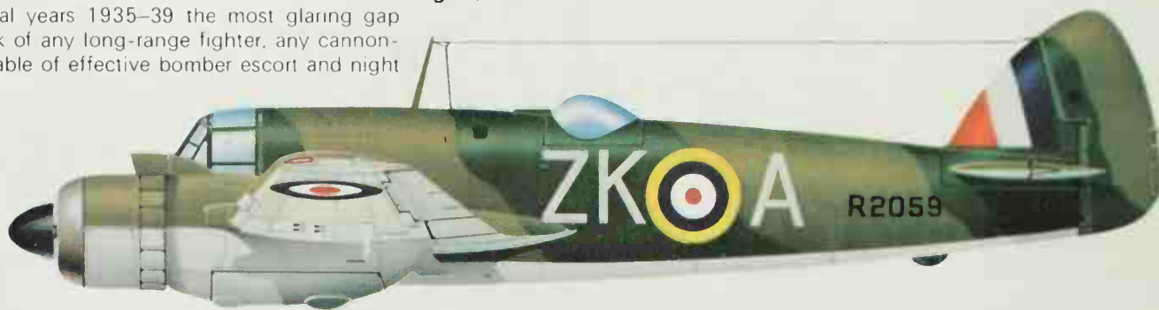
Above: Beaufighter TF.X with rear gun, radar and rocket rails.
