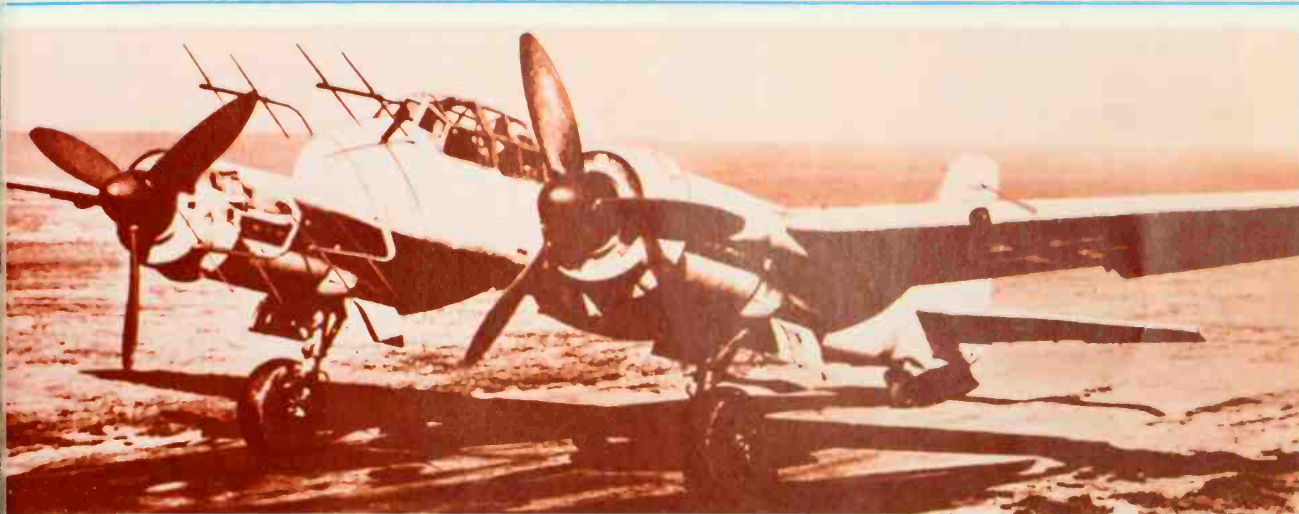
Above: One of the outstanding Ju 88 night fighters, the G-7a with Jumo 213 engines, Lichtenstein SN-2 FuG 220 radar and devastating armament.
