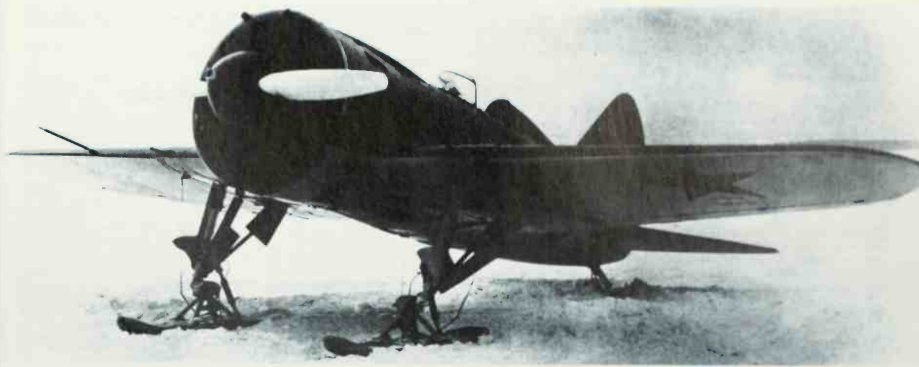
Above: Though this Type 24 is in Soviet summer camouflage it is wearing winter landing gear. The skis retracted flush under the fuselage.
