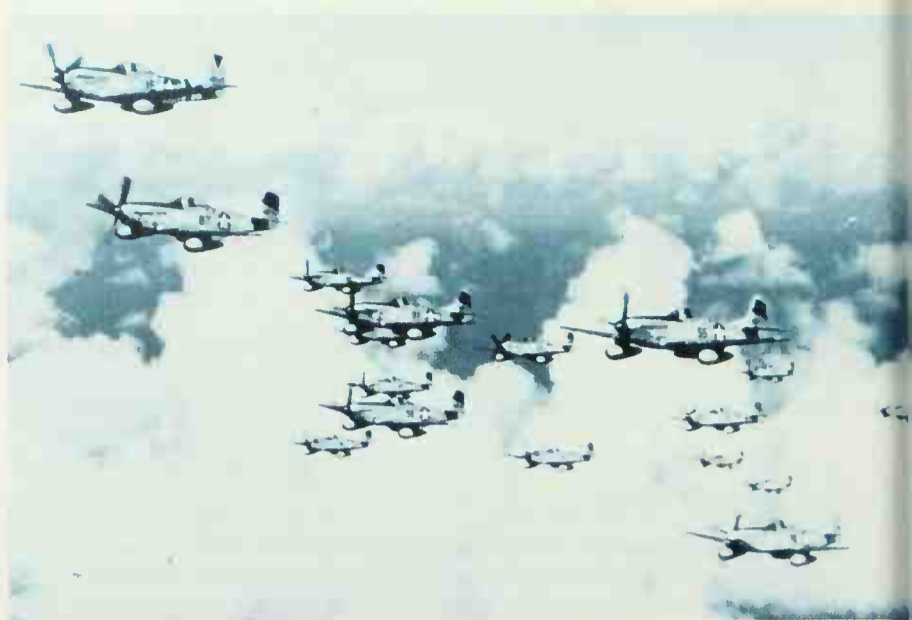
Above: A swarm of P-51D Mustangs, each with two 91.6-gal drop tanks, giving a range in excess of 2,000 miles. These examples served with the 15th Air Force in northern Italy.
