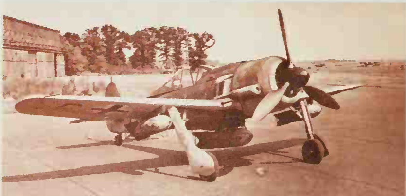
Above: This Fw 190A-5/U-13 has been modified to F-8 standard by MG 131 fuselage guns. It is carrying a 1,102lb and two 551lb bombs.
