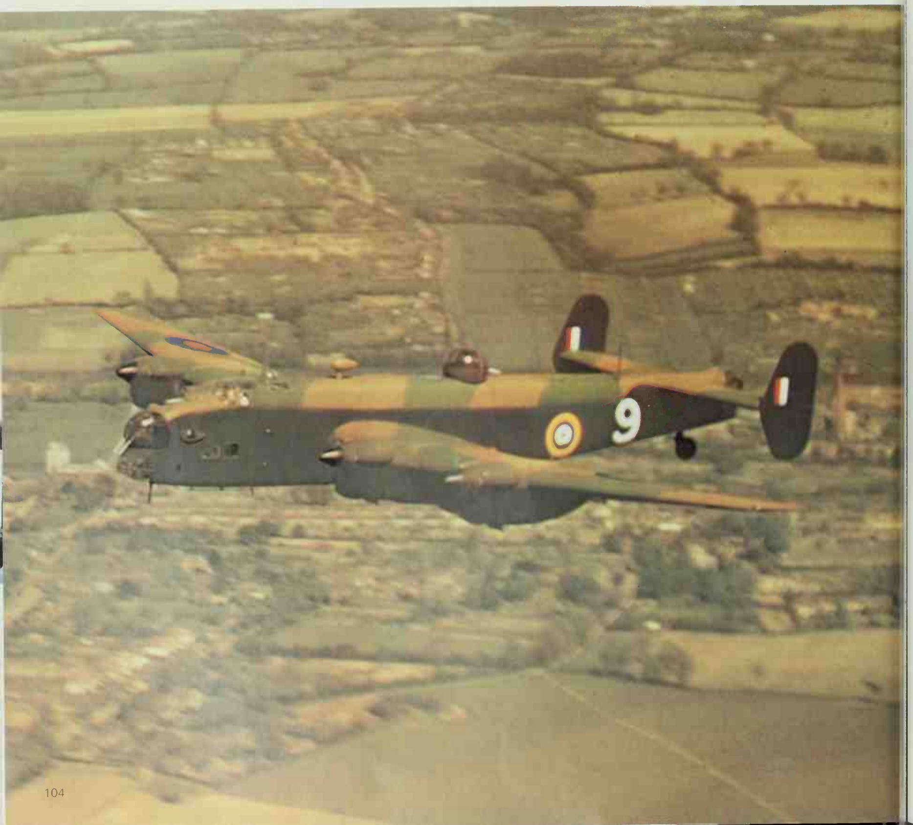
Below: An early Halifax II Series I with Boulton-Paul two-gun dorsal turret, on factory test.
