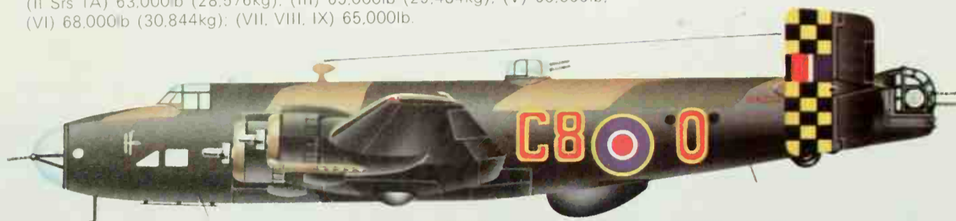
Below: An early Halifax II Series I with Boulton-Paul two-gun dorsal turret, on factory test.
