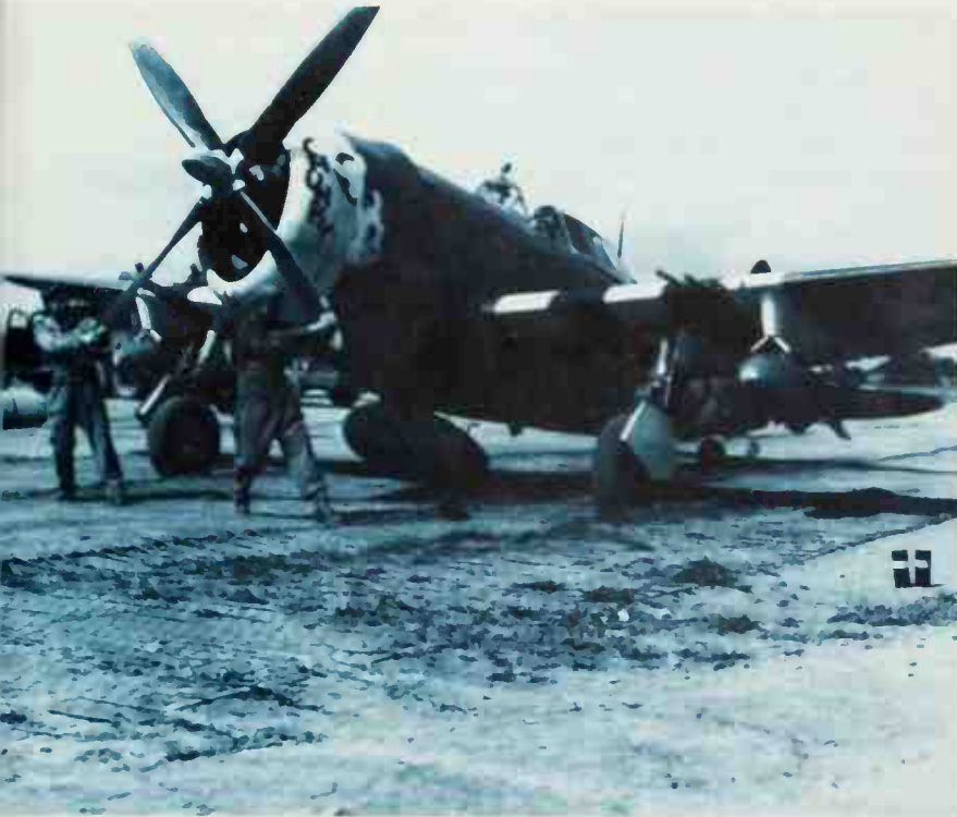
Above: When first used in Europe the P-47B was given white stripes to distinguish it from a Focke-Wulf 190 (which it in no way resembled). This P-47D-10 is seen later with Group insignia, D-day stripes, 108-gal paper tank and two 500lb bombs.
