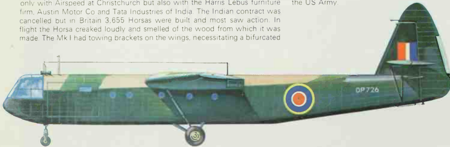
Left: DP726 was one of a batch of 100 Horsa I gliders built by the Austin Motor Company. It is depicted in normal training configuration, but on an operational mission was designed to jettison the entire main landing gears and alight on a large sprung ash skid under the centre fuselage.
