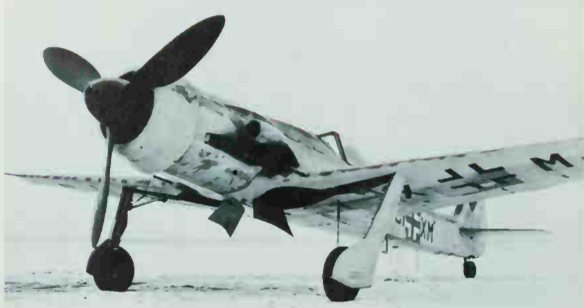
Above: The second production version of the Ta 152 was the C-series, without the long-span wing (photo shows Ta 152C V7, a Ta 152C-0/R11). This had a normal armament of one 30mm MK 108 and four MG 151 20mm, and flew in December 1944.
