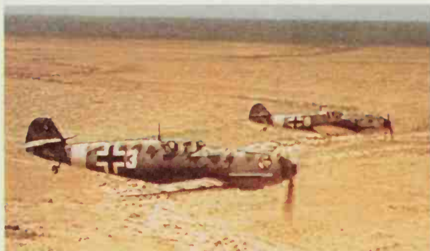
Above: Taken from a German propaganda film of 1941, this photograph depicts a pair of Bf 109E-4/Trop fighters of I/JG 27 flying over the Cyrenaican (Libyan) desert, soon after the entry of the Afrika Korps. Finish is 78 Light Blue, 79 Sand Yellow and 80 Olive Green, with the white tail band denoting the Mediterranean theatre of operations.
