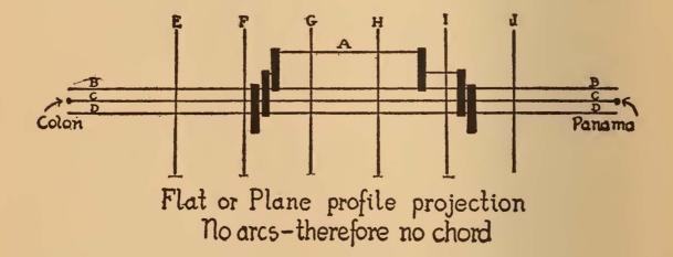
sents the high water line, C represents the mean sea level line, otherwise known as the horizontal datum line, and D represents the low water line; each line represents about fifty miles. The uppermost line
