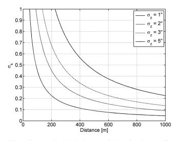
**Figure 2.** Standard deviation  $\sigma_k$  of the refraction coefficient as a function of the vertical angle accuracy  $\sigma_z$  and distance *S* between the stations.
