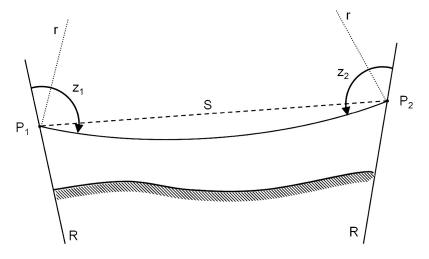
**Figure 1.** Measurement principle. Points  $z_1$  and  $z_2$  are vertical angle measurements, *S* is distance between endpoints, *R* is Earth radius, and *r* is refraction radius. Note that the path of light is bent toward the ground (negative refraction coefficient *k*), which is a typical situation for observations near the surface in the summer. The dashed line shows the unrefracted sighting between P<sub>1</sub> and P<sub>2</sub>.
