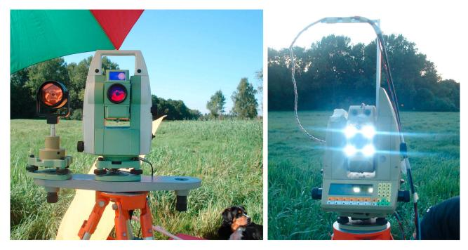
**Figure 3.** (left) Leica TCRP 1201+ tachymeter mounted together with a retroreflector on a ground plate. (right) Measurement system Daedalus: Leica TCA 1800 equipped with a light emitting diode target centered to the telescope.
