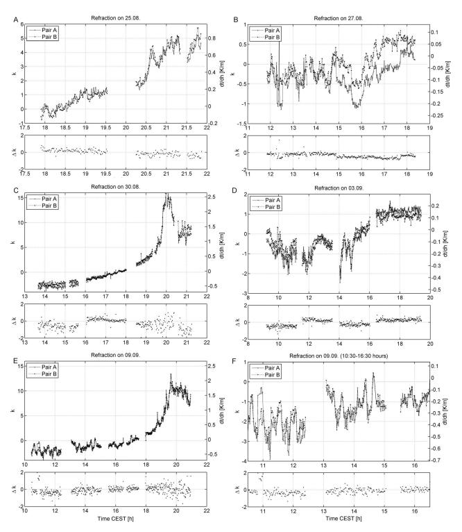
**Figure 5.** Complete results of refraction measurements using two pairs of TCRP total stations over five days: (a) 25 August 2008, (b) 27 August 2008, and (d) 03 September 2008 (cloudy days) and (c) 30 August 2008 and (e and f) 9 September 2008 (sunny days) along lines of sight A and B. The bottom part of each frame shows the difference  $\Delta k = k(\text{TCRP A}) - k(\text{TCRP B})$ .
