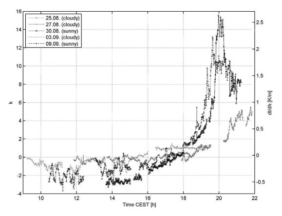
**Figure 7.** Refraction coefficients *k* on cloudy days (25 August 2008, 27 August 2008, and 03 September 2008) and sunny days (30 August 2008 and 9 September 2008). The displayed data are average values as observed along lines of sight A and B.
