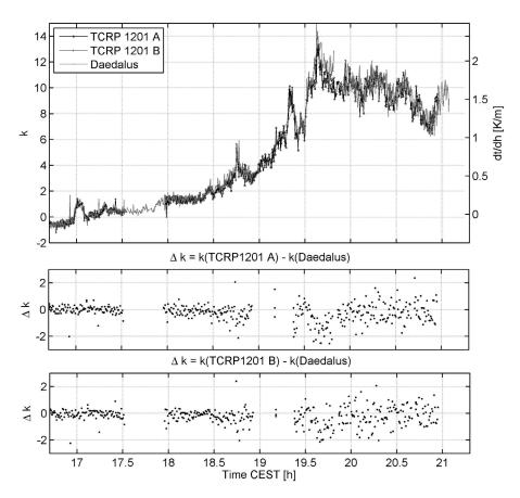
**Figure 6.** (top) Refraction coefficients *k* as observed with three pairs of tachymeters (TCRP 1201 A, TCRP 1201 B, and Daedalus) on 9 September 2008, (middle) difference  $\Delta k = k(\text{TCRP A}) - k(\text{Daedalus})$ , and (bottom) difference  $\Delta k = k(\text{TCRP 1201 B}) - k(\text{Daedalus})$ .
