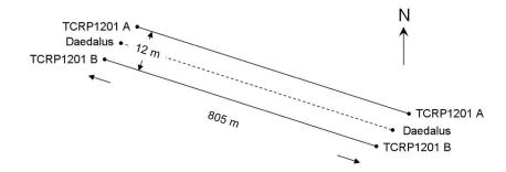
Figure 4. Arrangement of total stations for refraction measurement in test area Großmoor.
