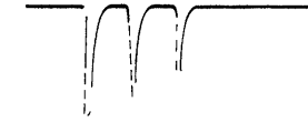
Fig. 16.4 Results of an echo experiment displayed on an oscilloscope. The first two pulses, which are separated by 137 ns, are the excitation pulses, and the third pulse is the echo. The first two photoelectric pulses have been attenuated to make all three of them comparable in size. (Reproduced from Abella, Kurnit and Hartmann, 1966.)
