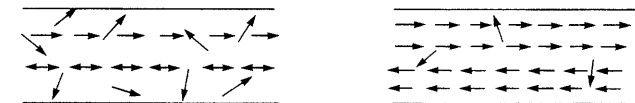
Fig. 18.2 Illustrating the growth of the stimulated emission probability with the intensity of the mode.
