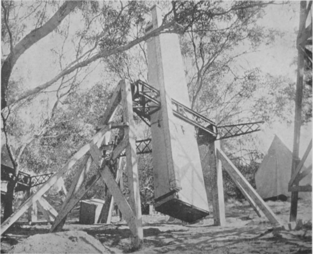
FIG. 8. Double astrograph, parallactically mounted, ( f = 450 cm, aperture 12 cm), as used by the Lick expedition (Lick I) in 1922 at Wallal, Australia, by CAMPBELL and TRUMPLER. (Photo: Lick Observatory.)
