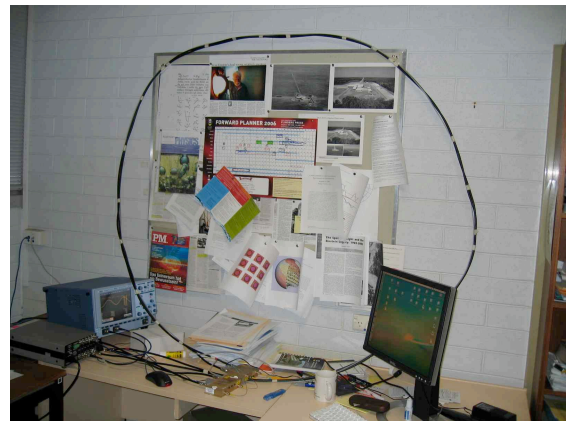
Fig. 13: The Flinders University Gravitational Wave Detector showing the cables formed into a loop. This configuration enables the calibration of the detector. The data from such a looping is shown in Fig. 14, but when the detector was relocated to an isolated underground laboratory.
