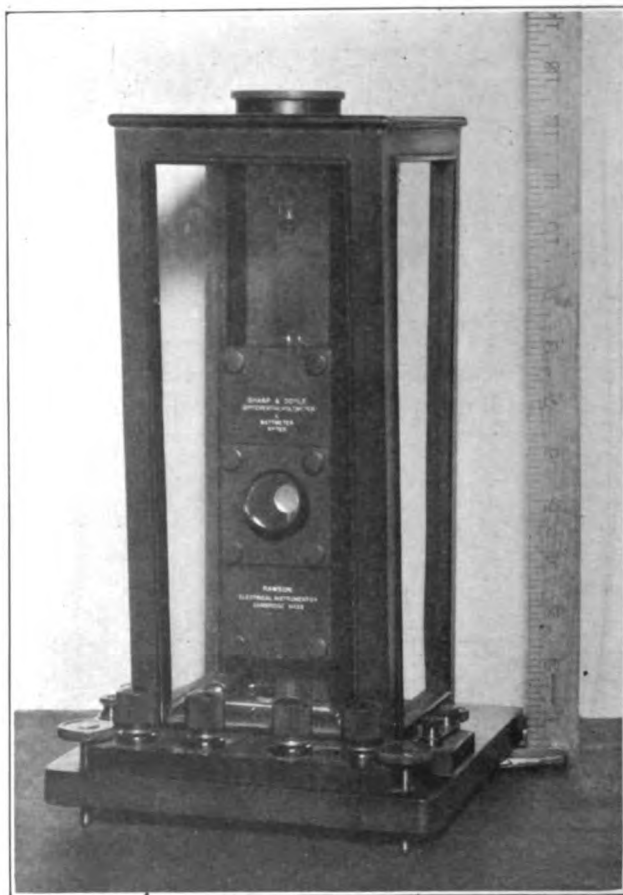
FIG. 4. Latest development of differential electro-dynamometer
