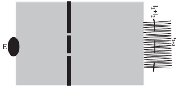
Figure 18.2 If the oscillations are too rapid, any probe (such as your eyes) would sense the average of I_{1+2} , the dotted curve I_1 + I_2 .
