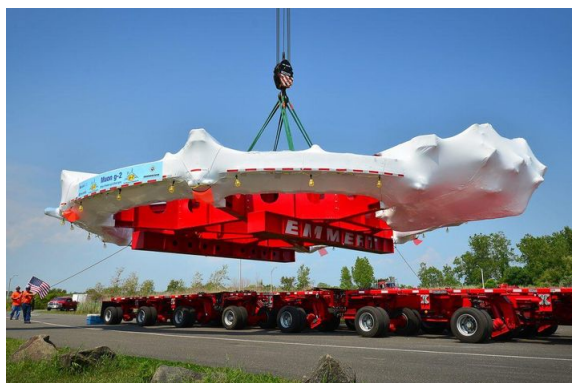
Fig. 9: Transportation of the 600 ton magnet to Fermilab
