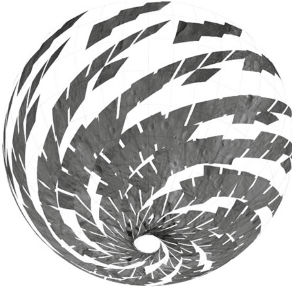
FIG. 16.21 : Ground track of the satellite Dawn. Upper: Reconstruction of the orbital elements by Ixion. The orbit denoted here by HAMO+ is at a slightly higher altitude than the one denoted by HAMO. Lower: The visible and infrared mapping spectrometer aboard NASA's Dawn spacecraft acquired this set of images during the high-altitude mapping orbit phase. Credit (image and caption) for the lower panel: NASA, JPL, Caltech, UCLA, ASI.
