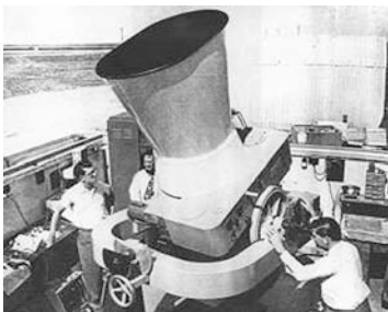
FIG. 6.5 : Baker–Nunn satellite tracking camera telescope. Installation at the Smithsonian Astrophysical Observatory (SAO) at the Woomera base in Australia in January 1958. Credit: NASA, Woomera Space Center.
