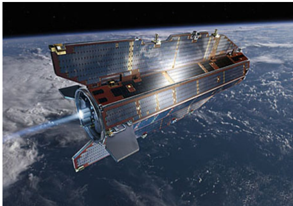
FIG. 3.7 : Artist's view of the satellite GOCE. The shape is designed to offer minimal resistance to atmospheric friction. The image shows the ions ejected by the drag compensation system. Credit: ESA.
