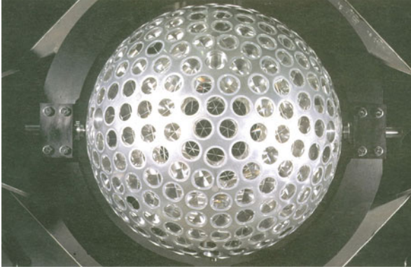
FIG. 3.8 : Preparation of LAGEOS-2. The satellite, of diameter 60 cm, is equipped with 426 reflectors (diameter 38.1 mm, depth 27.8 mm), made from cube corners whose 90^\circ angles are formed to an accuracy of 0.5 arcsec. Credit: Agenzia Spaziale Italiana (ASI).
