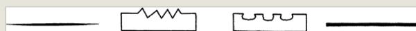
Fig. 4.2. Comparison of line profiles in engraving and etching. Left: engraved line and its profile, right: etched profile and resulting line.
