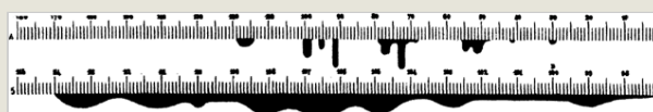
Fig. 2.22. Bunsen's symbolic plot of emission spectra and continuous spectra. The scale indicates readings from Bunsen's spectroscope, gauged at N_{\text{D}} = 50 at the abscissae of the black spots; their ordinates represent the intensity of the features. Woodcut. From Bunsen [1863 d ] pl. V, figs. 4-5.
