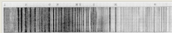
Fig. 6.2 Edmond Becquerel's extended spectrum including many newly discovered dark lines beyond the violet end of the visible spectrum. Copper engraving by Dulos. From E. Becquerel [1842a] plate, fig. 2 (note: the symbolic labels are not identical to the ones later adopted; cf. also Fig. 6.4).
