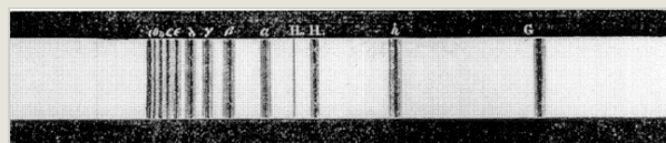
Fig. 8.2 Huggins's representation of the hydrogen series with twelve lines in the spectrum of \alpha Lyrae as a frequency plot (highest wavelength leftmost). Wood engraving. From Huggins [1879 b ] p. 270.
