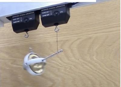
... that means the mass of the spinning part has been transferred over to the center of support. The data sheet shows that impressively clear: to the left we see that sensor1 and sensor2 are loaded with the respective weights of the ends of the system when *not* in precession, and when the system is allowed to precess at t=11.5s we see that the total mass of the system immediately is transferred to sensor 1.
