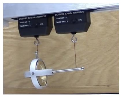
Then he burns away the thread supporting the spinning wheel, with the result of now W2 being equal to W(total) and W1 having become zero: W2 = W(total) with W1=0 ....
