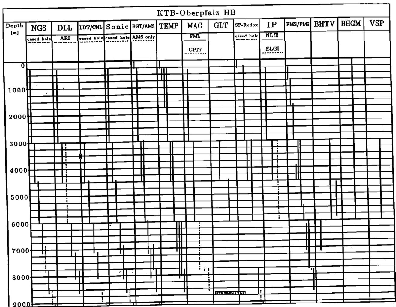
**Figure 3.** Summary of the major logging tools and their respective measuring interval in the superdeep hole. Abbreviations are NGS, natural gamma spectroscopy; DLL, electrical resistivity; sonic, seismic velocity; BGT, borehole geometry; TEMP, temperature log; MAG, magnetometer; GLT, geochemical logging tool; SP, self potential; IP, induction log; FMS/FMI, formation microscanner/formation microimager; BHTV, borehole televiewer; BHGM, borehole gravimeter; VSP, vertical seismic profiling.
