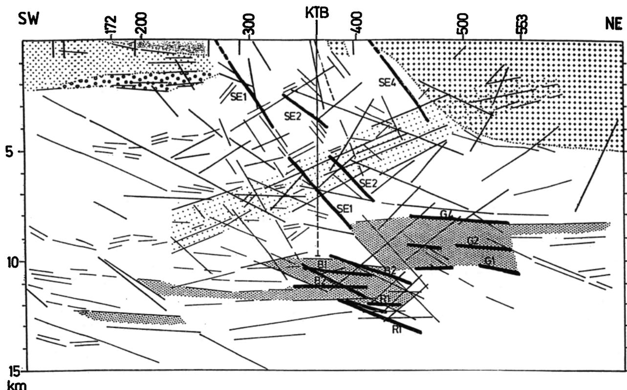
**Figure 5.** Interpretation of the seismic profile KTB 8502. Reflecting elements can be divided into two groups: steeply inclined reflectors (SE1-SE4) and subhorizontal reflectors (B, G, and R). The darkly shaded zone bounded by the subhorizontal reflectors is the "Erbendorf body."
