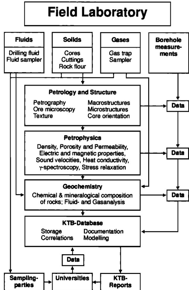
Figure 2. A flow chart showing the sampling and analysis scheme of the KTB field laboratory.
