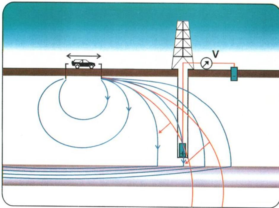
**Plate 4.** Schematic setup of the dipole-dipole experiment carried out at the final depth of 9101 m. Electric current was injected at variable distances from the drill site on two perpendicular profiles. The electrical field was measured by two probes at the bottoms of the superdeep hole and the pilot hole. The first results confirm that the superdeep hole penetrated into the high-conductivity layer predicted to lie at  $10 \pm 1$  km (shaded band).
