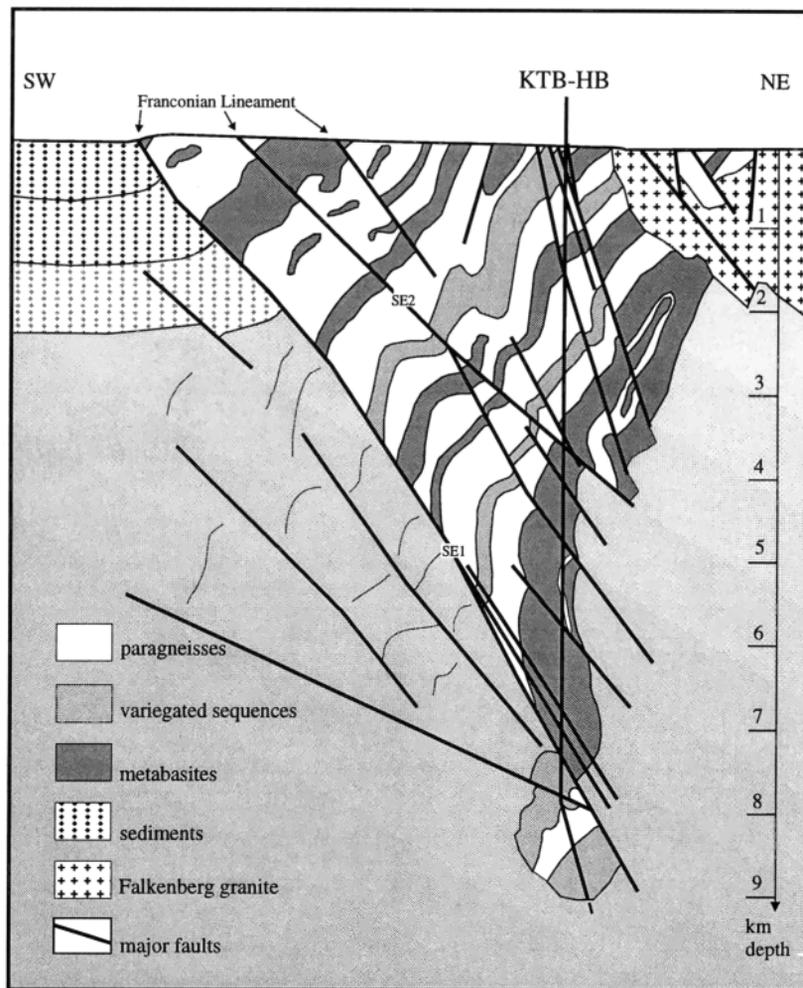
**Figure 4.** Schematic SW-NE profile through the ZEV in the surroundings of the KTB site (no vertical exaggeration). The metamorphic sequence of the ZEV has a polyphase history, with early high-pressure metamorphism at about 475 Ma, and later, Barrovian-type metamorphism at about 400-375 Ma. The Falkenberg granite, to the NE, intruded at about 310 Ma. To the SW are foreland sedimentary sequences of Upper Cretaceous, Triassic, and Permo-Carboniferous ages.
