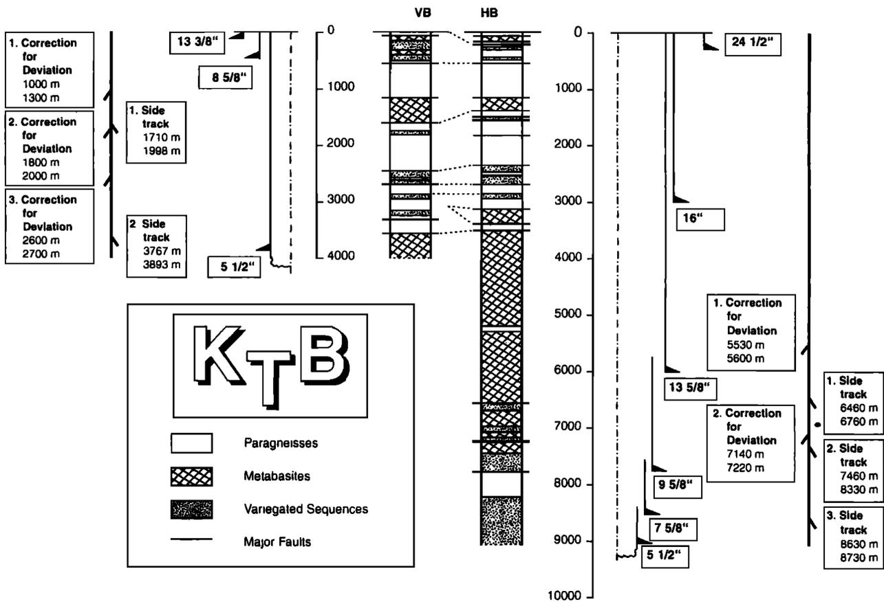
**Figure 1.** An outline of the final borehole configuration, showing the side tracks and corrections for deviation, casing scheme and lithological profile of (left) the pilot hole and (right) the superdeep hole.
