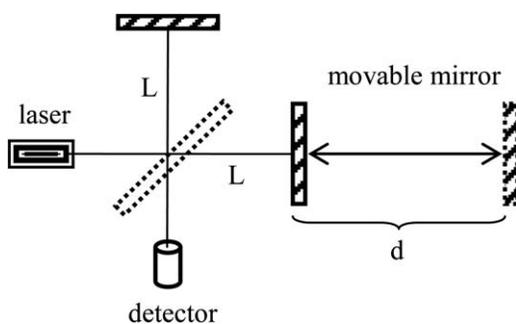
FIG. 1. Michelson interferometer as a length comparator.
