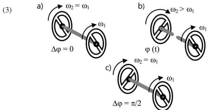
FIG. 2. (a) Two rigidly coupled wheels rotating in phase at frequency  $\omega_1$ . (b) Wheel 2 decoupled from 1 and rotating at a higher frequency  $\omega_2$ . (c) Both wheels coupled again after a phase shift of  $\Delta\phi = \pi/2$ .
