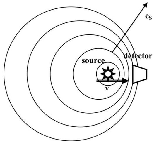
FIG. 4. Doppler effect with moving source.
