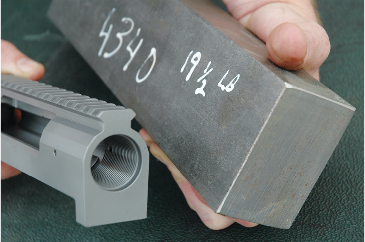
Surgeon magnum actions are milled to fly-wing tolerances from rectangular steel billets. The integral rail is sloped to add elevation "gain" for long shooting.
