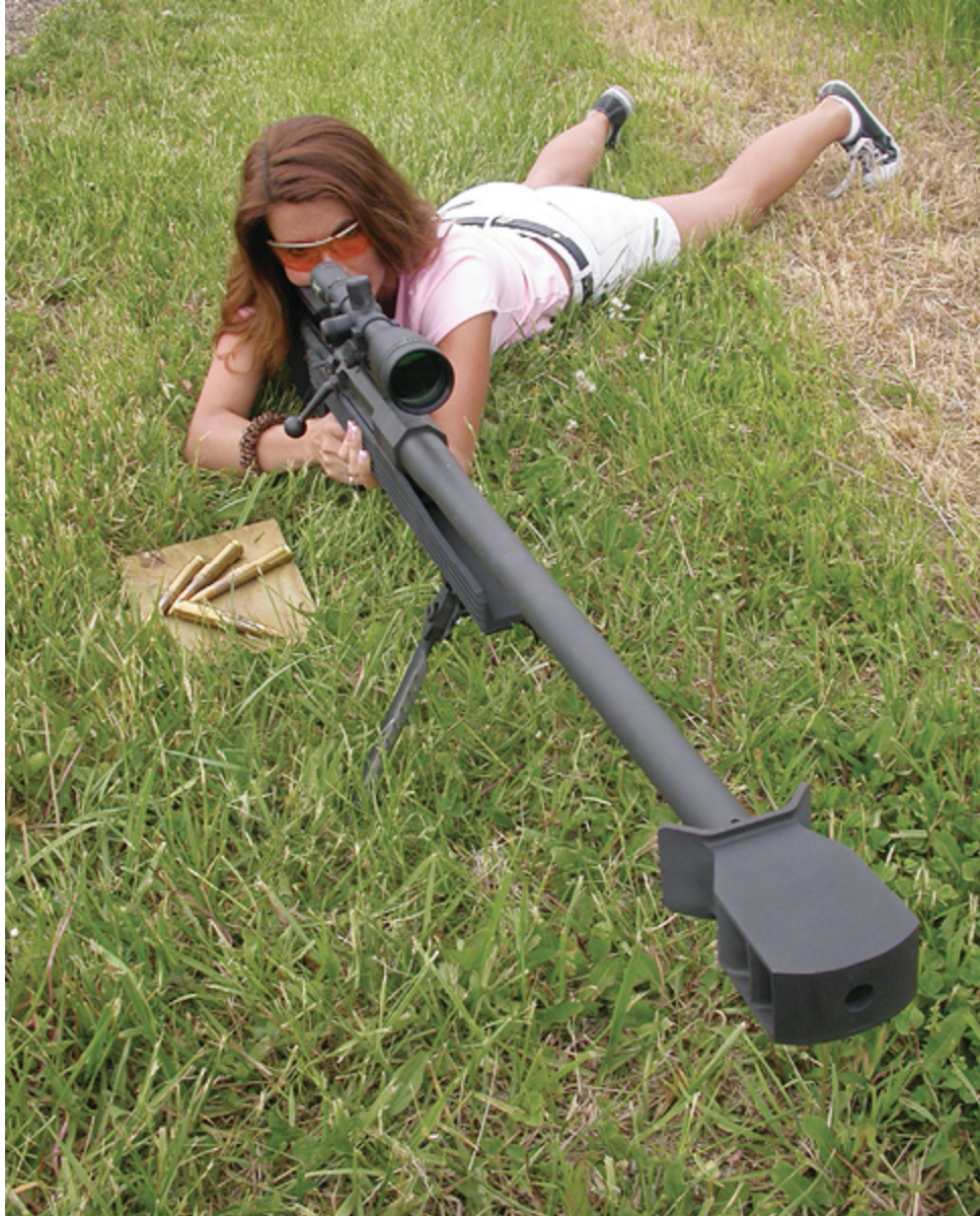
A big brake, sturdy bipod, and heavy rifle make even the .50 BMG manageable by petite shooters.
