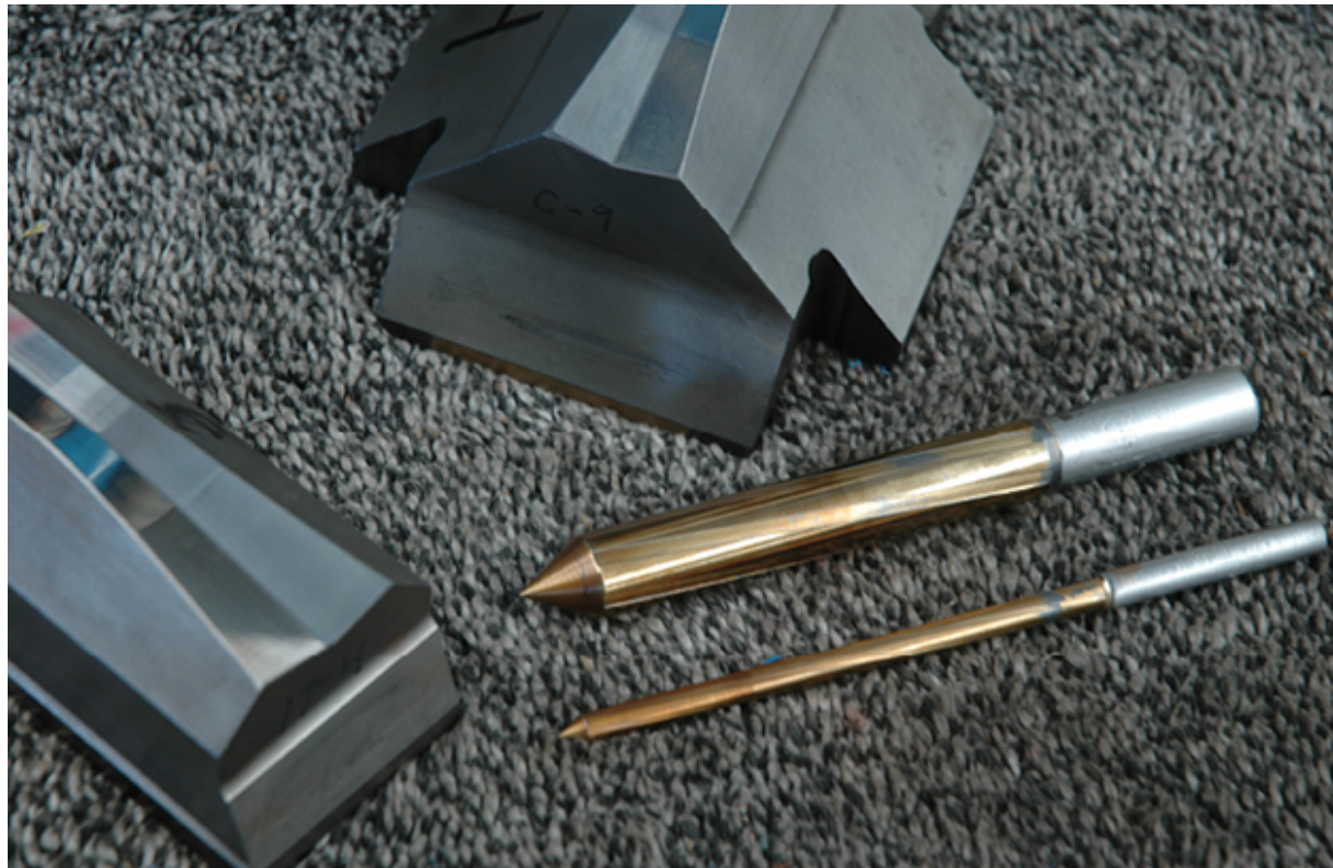
Hammers flank two rifling mandrels on a bench near a Ruger hammer-forging machine.
