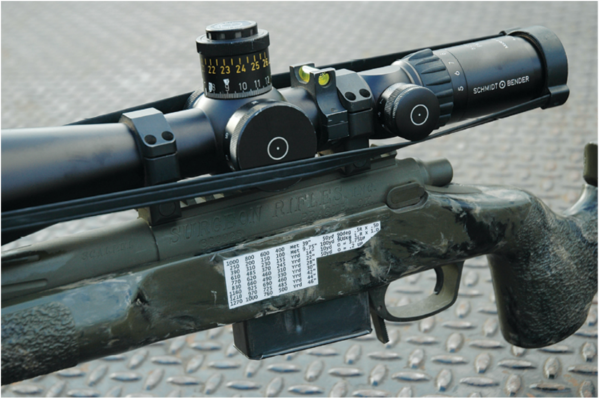
Taping drop data to your rifle puts it always within easy reach. Here, a Surgeon Scalpel.
