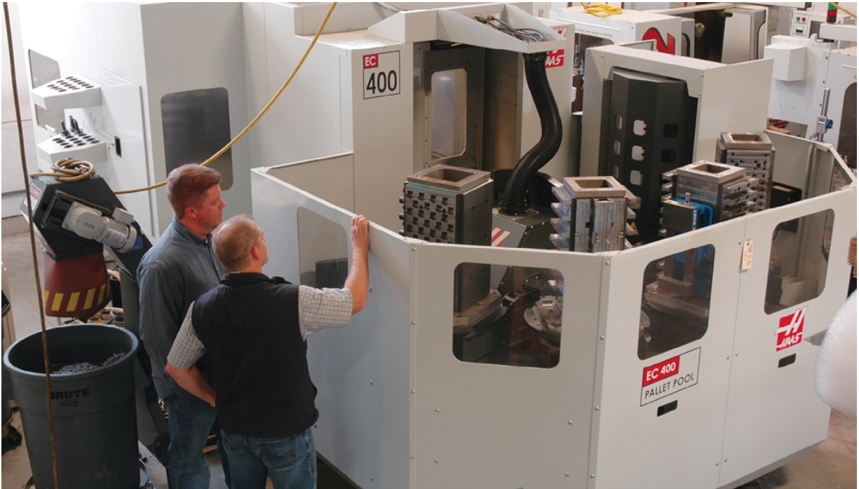
This modern CNC center at Montana Rifle Company produces finished rifle actions.
