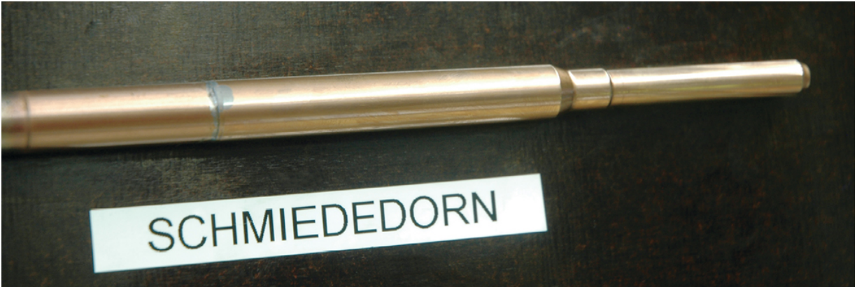
This Blaser hammer-forging mandrel includes the chamber, as well as the rifling.
