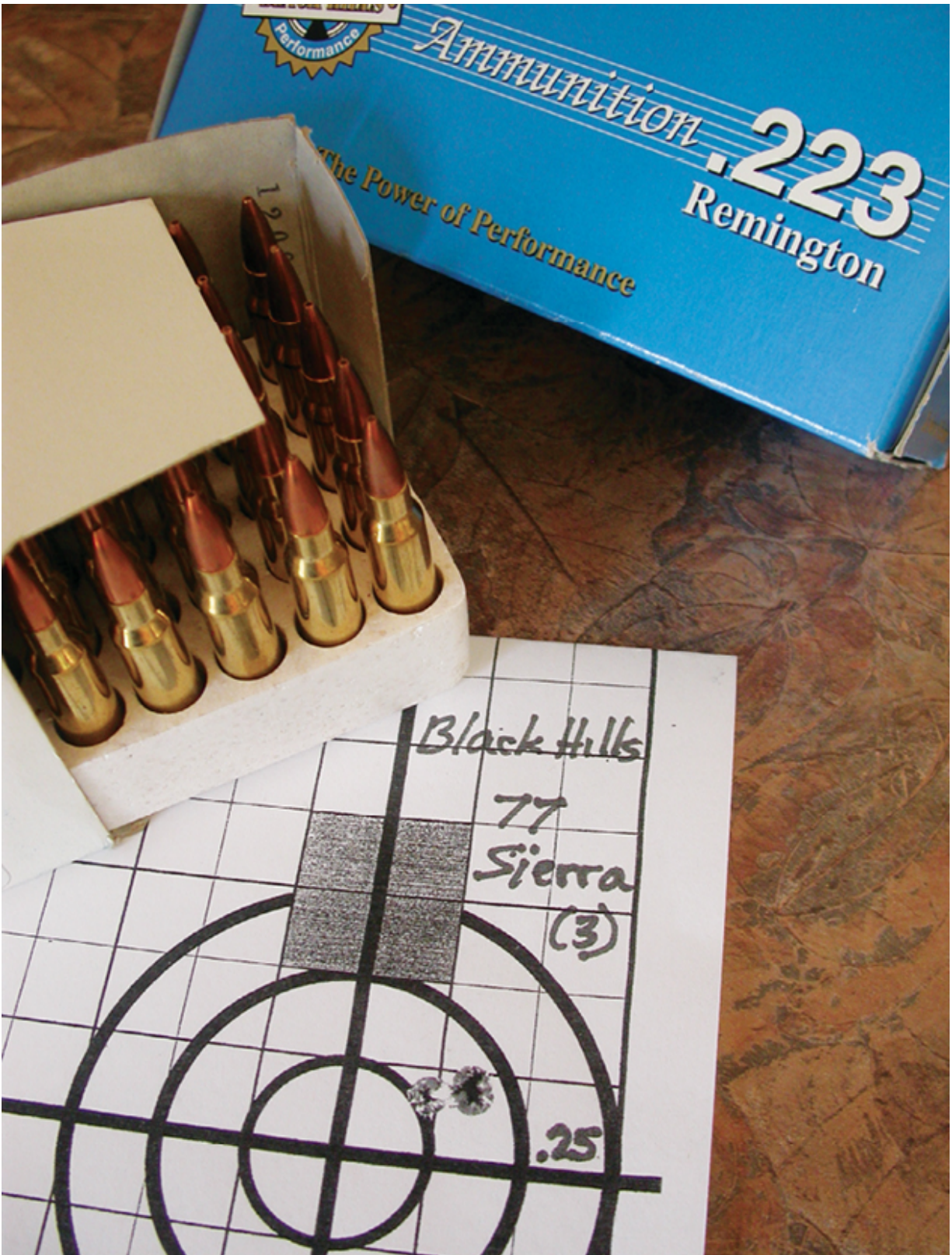
Relatively steep rifling pitch is needed to produce group like this with heavy .223 bullets.
