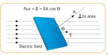
**Gauss law** states the total flux linked with a closed surface is  $1/\epsilon_0$  times the charge enclosed by the closed surface.
