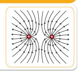
**Electric flux** is the rate of flow of the **electric** field through a given area. Electric flux in an area is the **Electric field** multiplied by the **area** of the surface projected in a plane **perpendicular** to the field.
