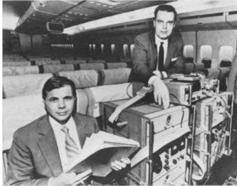
The experiment consisted in using two high precision Caesium atomic clocks, synchronised with a US reference ground station (USNO) for flying them on commercial aircrafts for two separated closed flight trips, one eastward, and one westward. After returning to USNO the clock times were compared with the reference time and the time shifts recorded. The observations were compared with the predicted values calculated applying the general relativity formula and a close matching was found.
