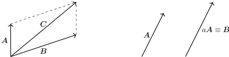
Figure C.1 Prototype properties of vectors: Vector addition and scalar multiplication.
